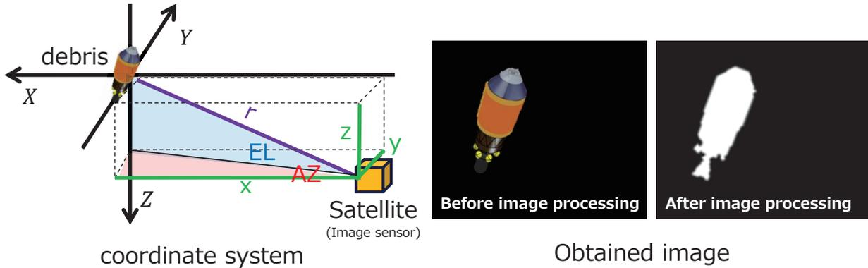
In this method, debris is captured using sunlight and albedo with visible light camera. Relative position( $r, x, y, z$ ), Azimuth(AZ), Elevation(EL) is obtained by performing image processing on the acquired image.
