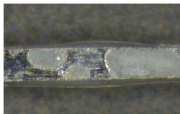
Fig.5. Close-up view of gate electrode coated with PFA.
