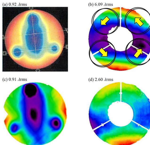
**Figure 3.** (a) SFE map of the ACF with a designed large deformation. (b) The WFE map of the telescope obtained by the sub-aperture stitching measurement using the deformed ACF, shown together with the positions and directions of the small movements of the ACF. (c) The SFE map of the ACF reproduced by our method. (d) The resultant WFE map of the telescope obtained by the sub-aperture stitching measurement after the correction of the ACF errors.
