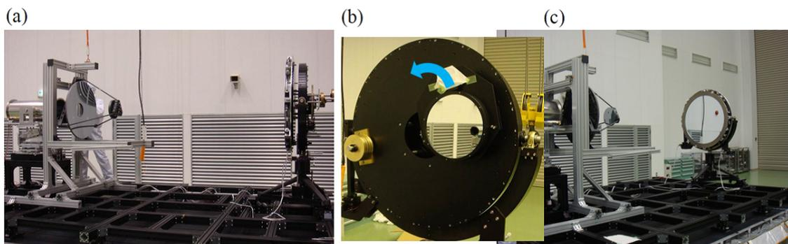
**Figure 1.** (a) Configuration for the sub-aperture stitching measurement. The telescope and interferometer are set on the left-hand side, while the 300-mm ACF is set on the right-hand side. (b) The 300-mm ACF used in the sub-aperture stitching measurement. The ACF is rotated by a step angle of 22.5 degrees in a counterclockwise direction. (c) Configuration for the full-aperture measurement. The 900-mm flat mirror is placed on the right-hand side.
