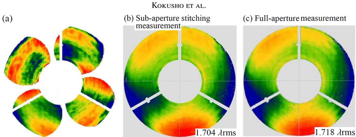
**Figure 2.** (a) Sub-aperture WFE maps at four radial positions. (b) The WFE map of the telescope obtained by stitching the sub-aperture datasets. (c) The WFE map of the telescope obtained by the full-aperture measurement using the 900-mm ACF.
