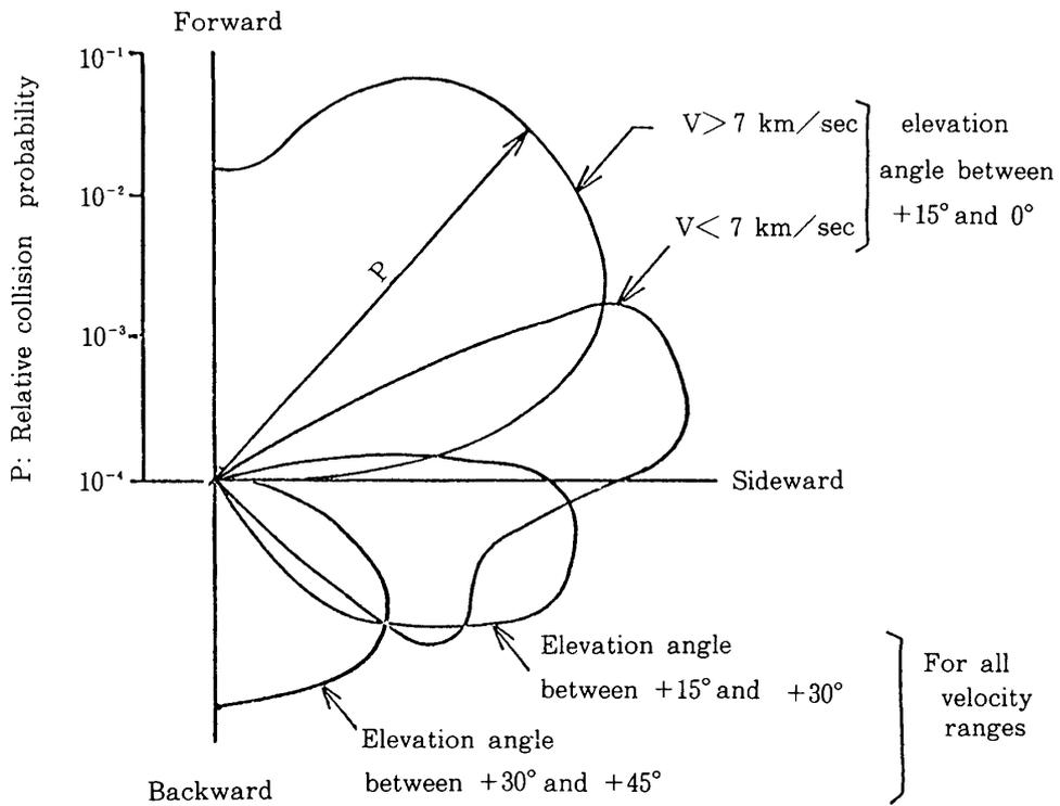
Fig. 9b. Directional Collision Probability Projected on Local Horizontal Plane
