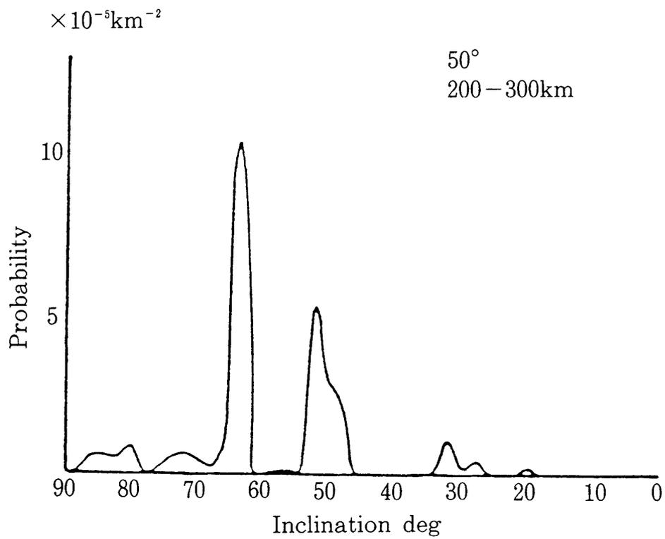
Fig. 5. Contribution of Orbital Inclination to Collision Probability
