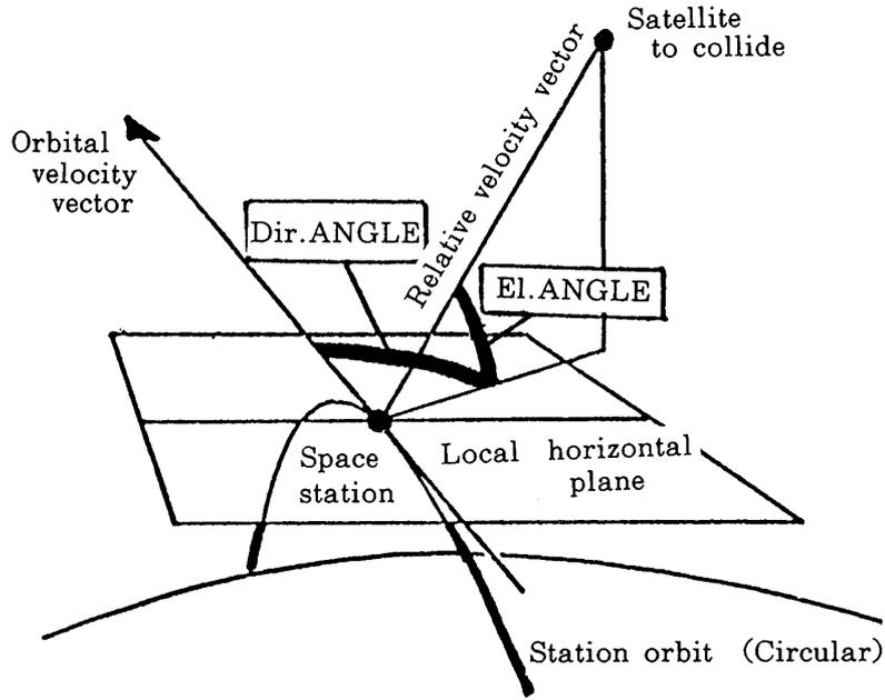
Fig. 9a. Coordinate System for Search Radar
