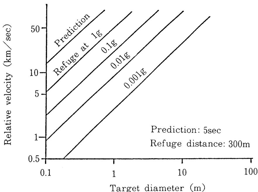
Fig. 10. Required Acceleration Level for Refuging Maneuver
