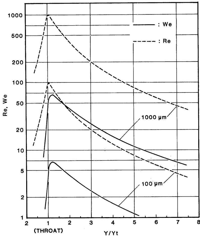
Fig. 3-10. Variation of Weber number and Reynolds number in the nozzle. Flow model: PFFM.
