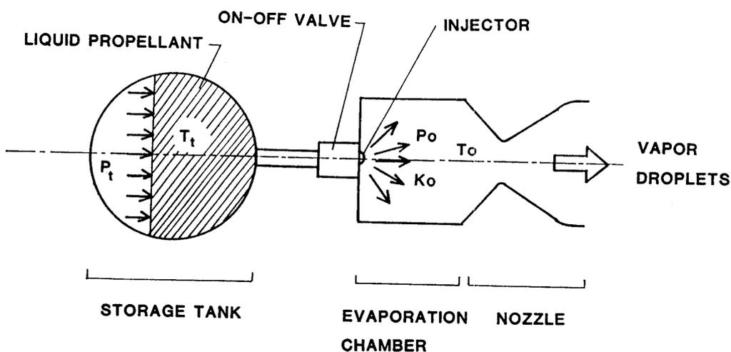
Fig. 1-3. Conceptual model of spray thruster.
