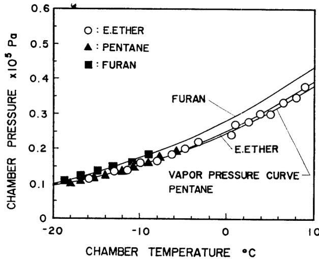
Fig. 2-8. Pressure-temperature characteristic in the evaporation chamber.
