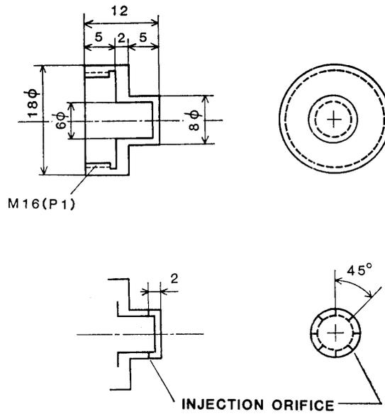
Fig. 2-2. Injector configuration.
