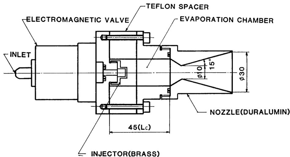
Fig. 2-1. Schematic configuration of spray thruster type-1.
