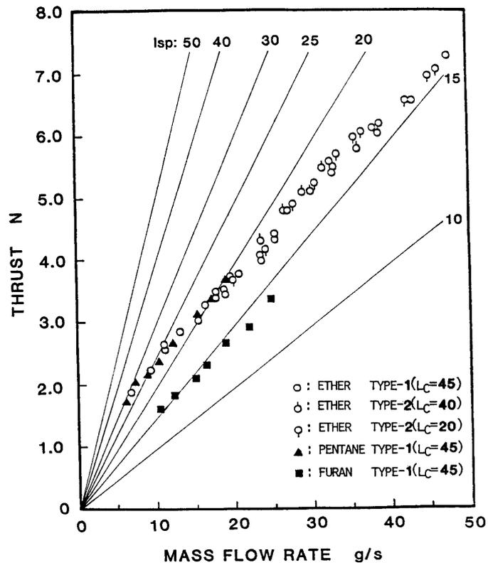
Fig. 2-10. Thrust vs. mass flow rate.
