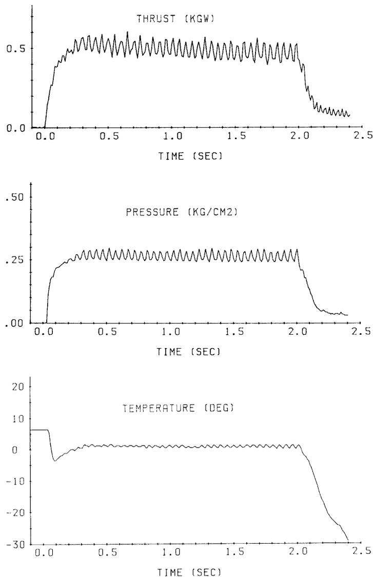
Fig. 2-7. Response characteristics of thruster type-2, feed pressure: 0.25 MPa.
