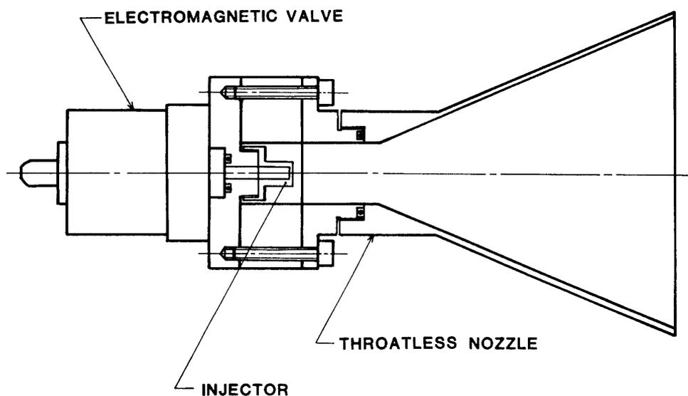
Fig. 4-9. Schematic configuration of throatless nozzle.
