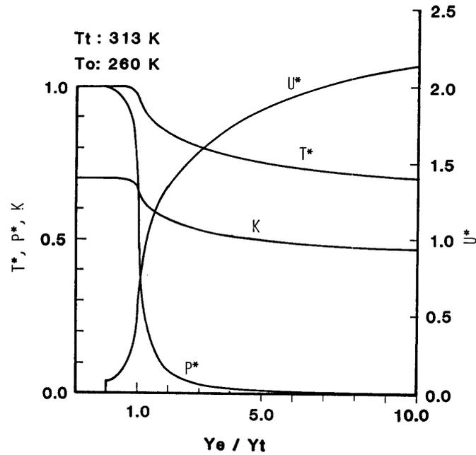
Fig. 3-2. Flow structure in EFM,  $T_t=313\text{K}$ ,  $T_o=260\text{K}$ .
