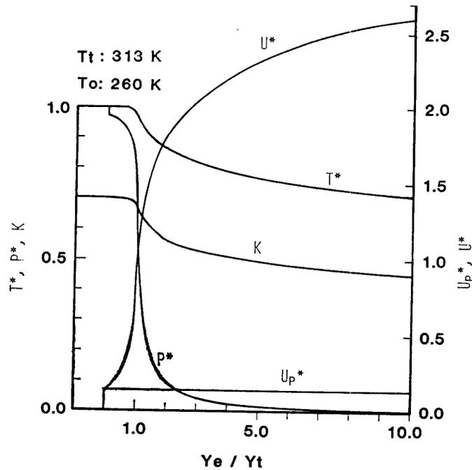
Fig. 3-6. Flow structure in PFFM,  $T_t=313\text{K}$ ,  $T_o=260\text{K}$ .
