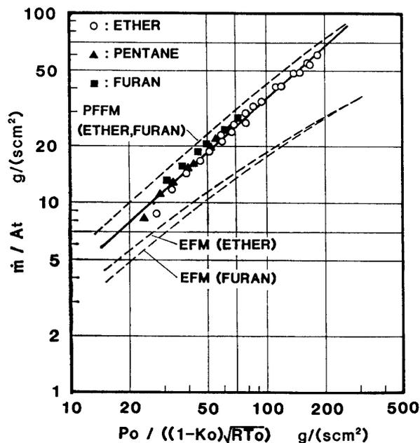
Fig. 4-1. Comparison of experimental results with numerical ones: characteristics of mass flow rate density.
