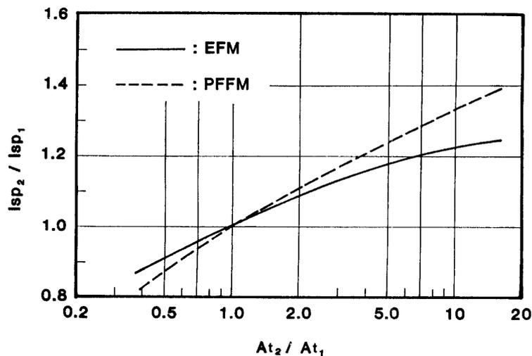
Fig. 4-8. Effect of nozzle dimension on the  $I_{SP}$ .
