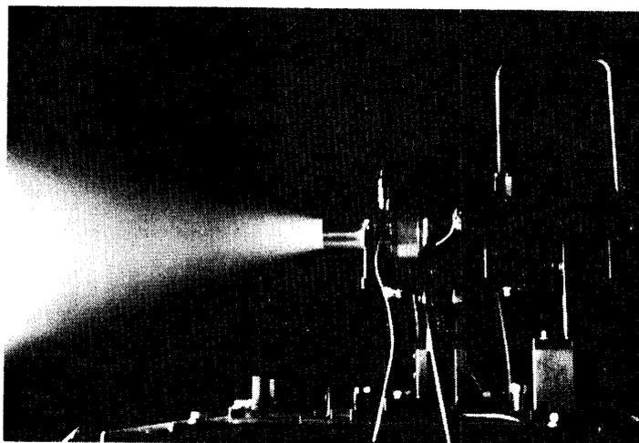
Fig. 2-13. Photograph of spray thruster in operation, mass flow rate: 25 g/sec.
