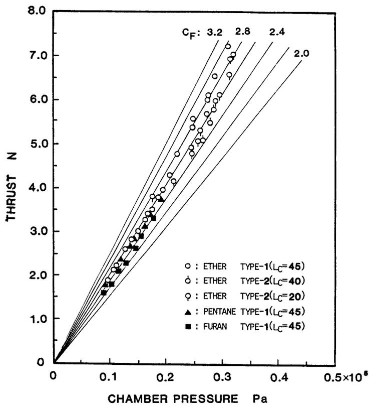
Fig. 2-12. Thrust vs. chamber pressure.
