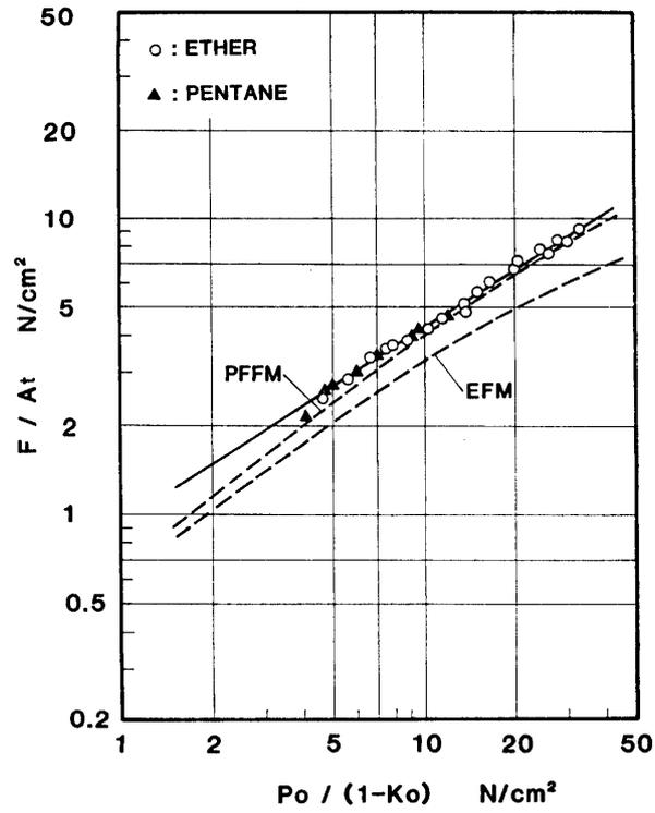
Fig. 4-2. Comparison of experimental results with numerical ones: characteristics of thrust density.
