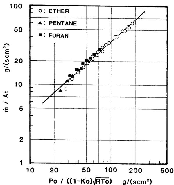
Fig. 2-15. Characteristics of mass flow rate density.
