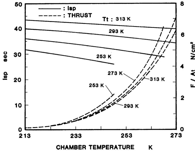
Fig. 4-10. Effect of operational temperature on the thrust performance.
