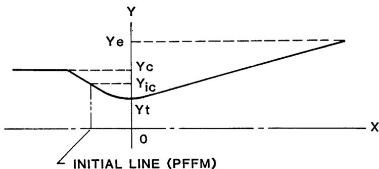
Nozzle configuration for numerical calculation.
