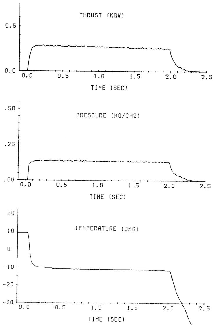
Fig. 2-6. Response characteristics of thruster type-1, feed pressure: 0.29 MPa.
