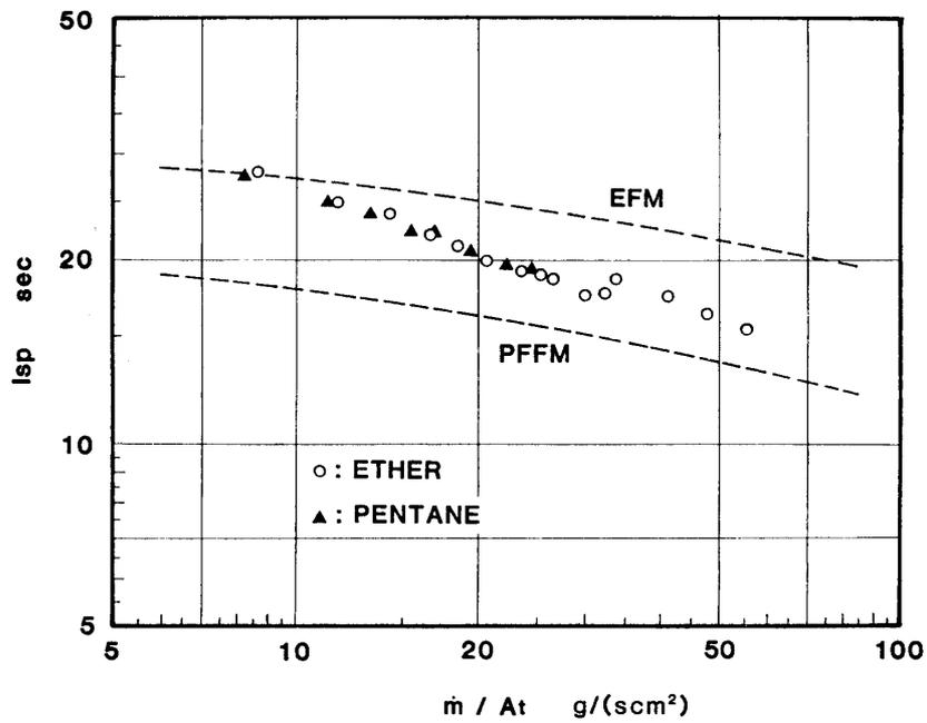
Fig. 4-3. Comparison of experimental results with numerical ones: characteristics of specific impulse.
