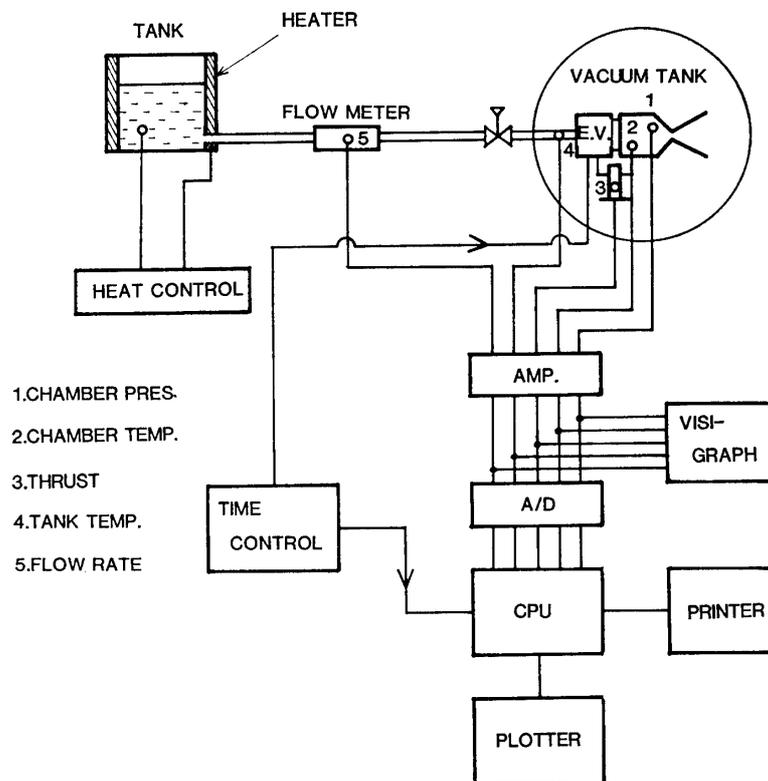
Fig. 2-4. Measurement system.
