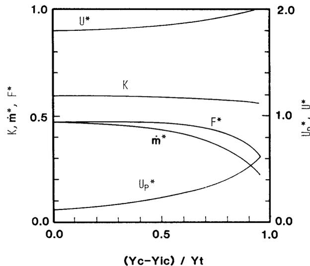
Fig. 3-5. Effect of the position of initial line on the flow structure at expansion ratio of 9.
