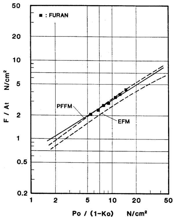
Fig. 4-4. Comparison of experimental results with numerical ones: characteristics of thrust density for Furan.
