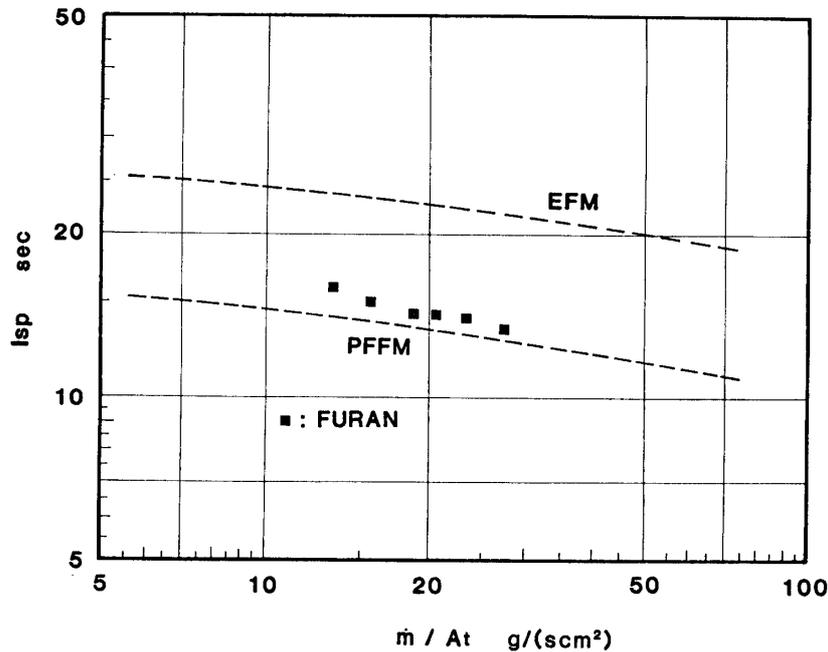
Fig. 4-5. Comparison of experimental results with numerical ones: characteristics of specific impulse for Furan.
