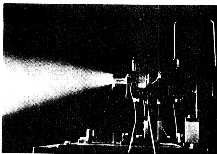
Fig. 2-14. Photograph of spray thruster in operation, mass flow rate: 42 g/sec.
