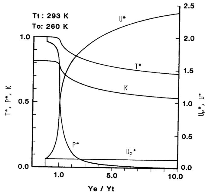
Fig. 3-7. Flow structure in PFFM,  $T_t=293\text{K}$ ,  $T_o=260\text{K}$ .
