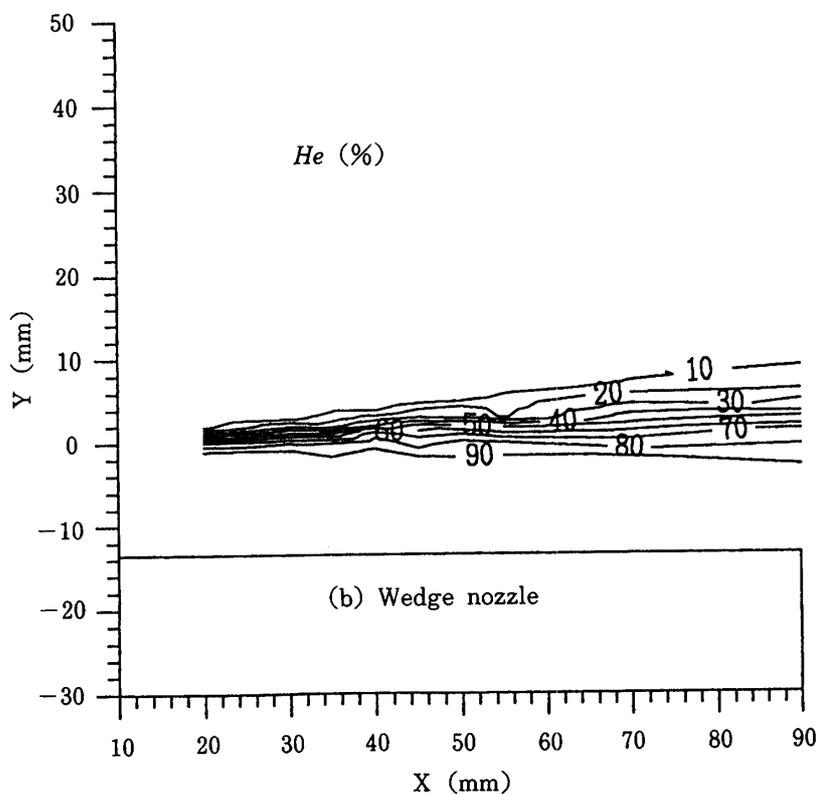
Fig. 9. Contour of concentration ratio of helium for the flow in Case 1 (in (a)), Case 2 (in (b)) and Case 3 (in (c)).
