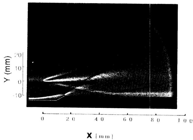
Fig. 4. Schlieren photographs for different nozzle configurations of Case 1 (in (a)), Case 2 (in (b)) and Case 3 (in (c)).
