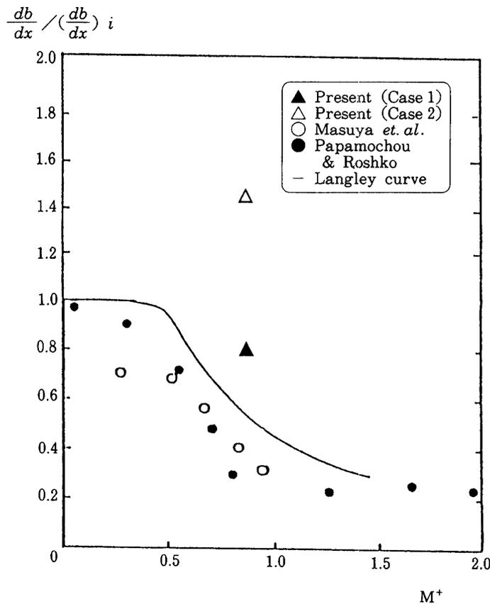
Fig. 11. Normalized growth rate of the mixing layer versus the compressibility factor  $M^+$ . The  $(db/dx)_i$  is the growth rate without the compressibility effect.
