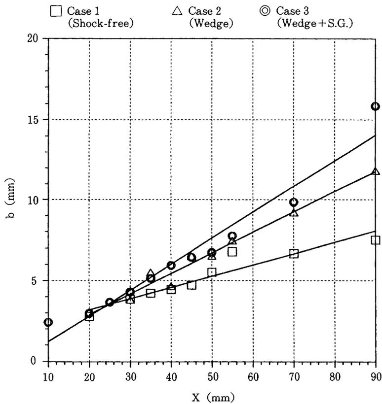
Fig. 10. Variation of mixing layer width along the stream direction (x coordinate).
