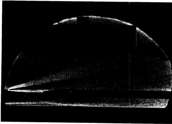
Fig. 6. Schlieren photography of the flow field for the Case 1 when the sampling probe is inserted.
