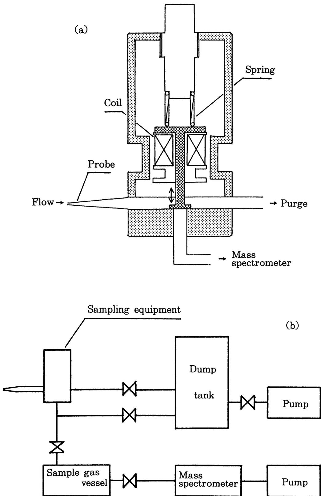
Fig. 5. Schematic figures of the sampling equipment (in (a)) and the probe (in (b)).
