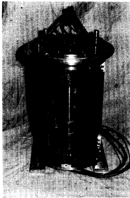
図6 よじれ戻し軸受
