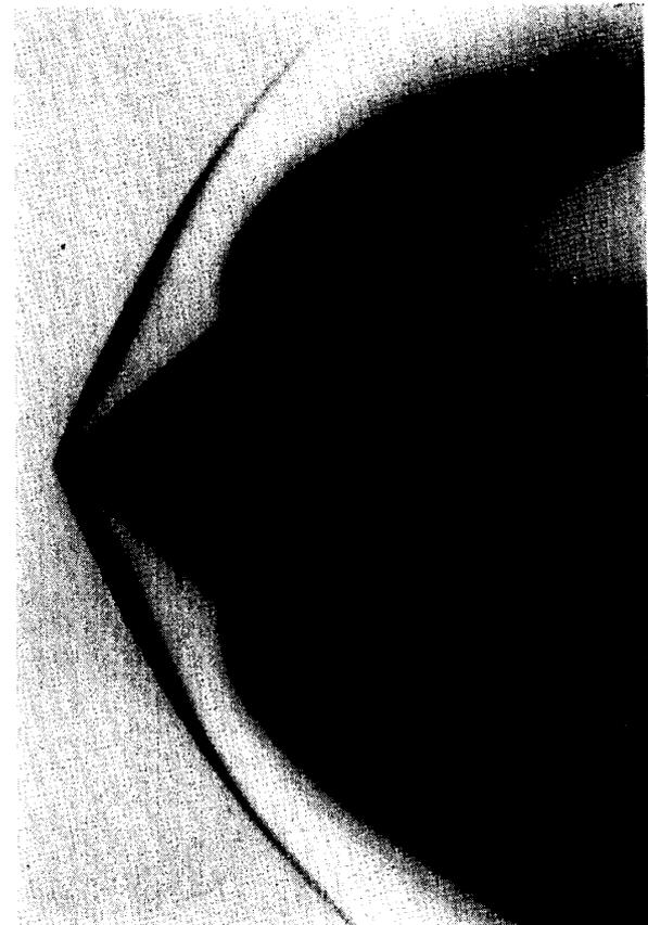
FIG. 10. Schlieren photograph of a limiting flow field.  $M=2$ ,  $\delta=40.57^\circ$ .
