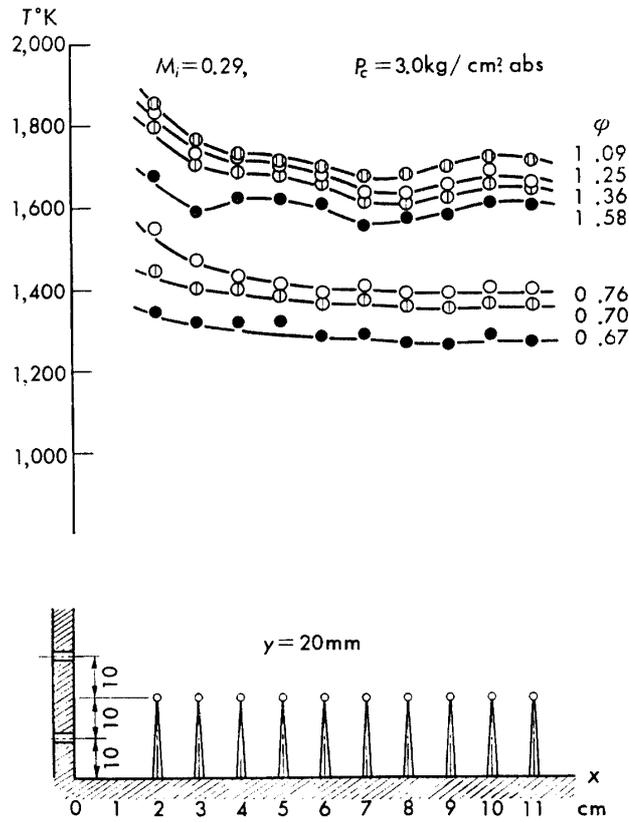
FIG. 18. Distribution of mean gas temperature in reaction zone;  $P_c = 3.0 \text{ kg/cm}^2 \text{ abs.}$ ,  $M_i = 0.29$ ,  $y = 20 \text{ mm}$ .
