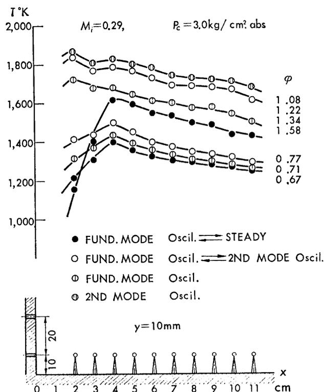
FIG. 16. Distribution of mean gas temperature in reaction zone;
