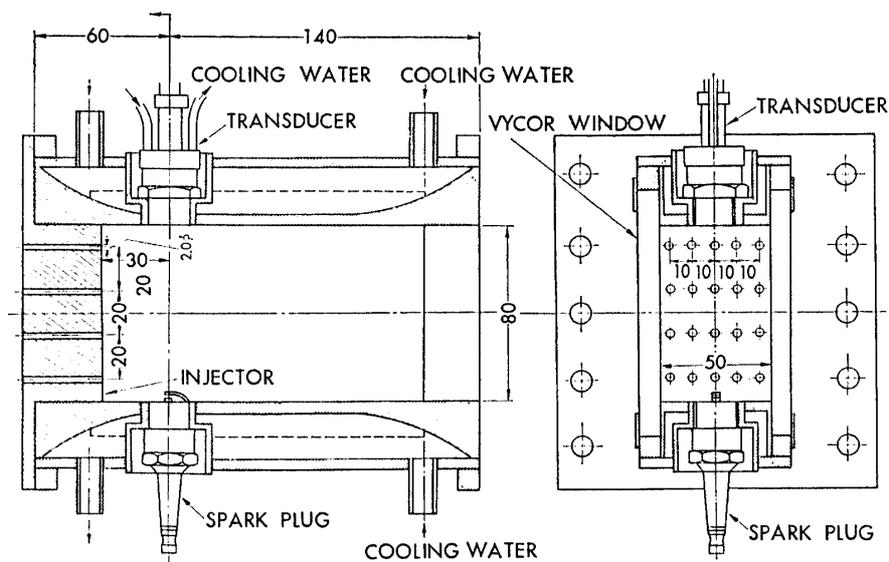
FIG. 3. Combustion chamber section for photographic study of reaction zone at atmospheric chamber pressure.
