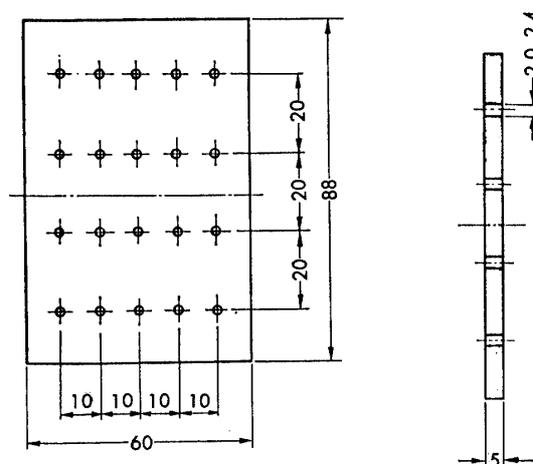
FIG. 2. Specifications for injector plates.
