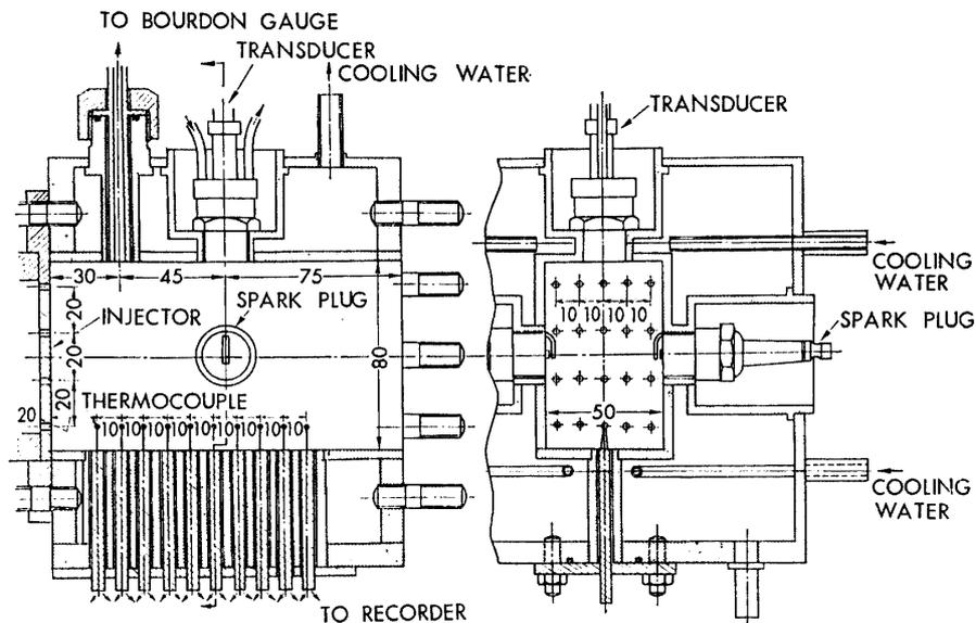
FIG. 4. Combustion chamber section for measurement of temperature distribution in reaction zone.
