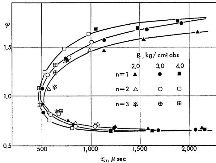
FIG. 10. Effect of combustion chamber pressure on critical oscillation period;  $M_i=0.29$ .
