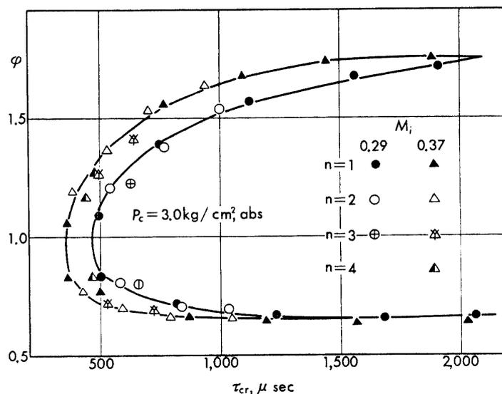
FIG. 14. Effect of injection Mach number on critical oscillation period;  $P_c = 3.0 \text{ kg/cm}^2 \text{ abs}$ .
