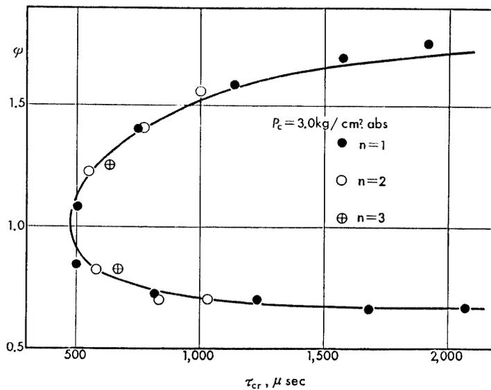
FIG. 9. Effect of injection section length on critical oscillation period.
