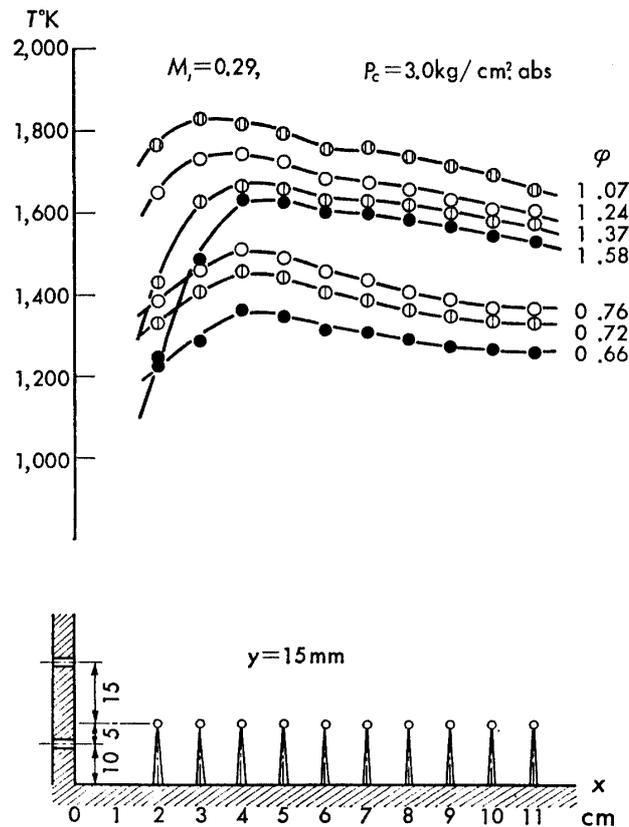
FIG. 17. Distribution of mean gas temperature in reaction zone;
