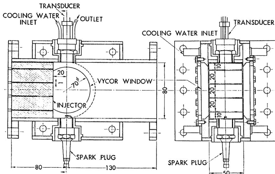
FIG. 5. Combustion chamber section for photographic study of reaction zone during oscillative combustion.
