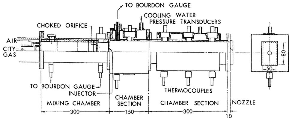
FIG. 1. Research rocket motor.
