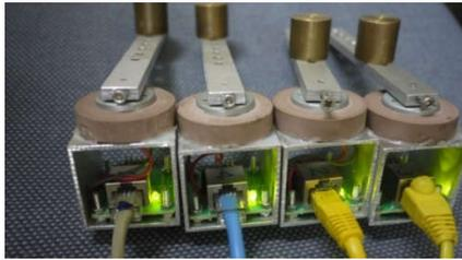
Photograph 3. Hoop generator and sensor. The amplified generator and gravitational acceleration outputs were transmitted via a LAN cable.
