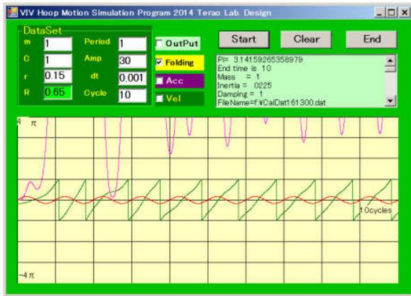
Figure 7. Sample of a diverging motion appeared in the hoop weight roll angle. The roll angle is shown from  $-\pi$  to  $\pi$ .
