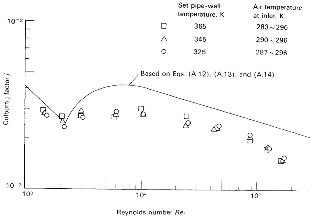
FIG. 15. The Colburn  $j$  factor for heat transfer as a function of the Reynolds number of the air flow.
