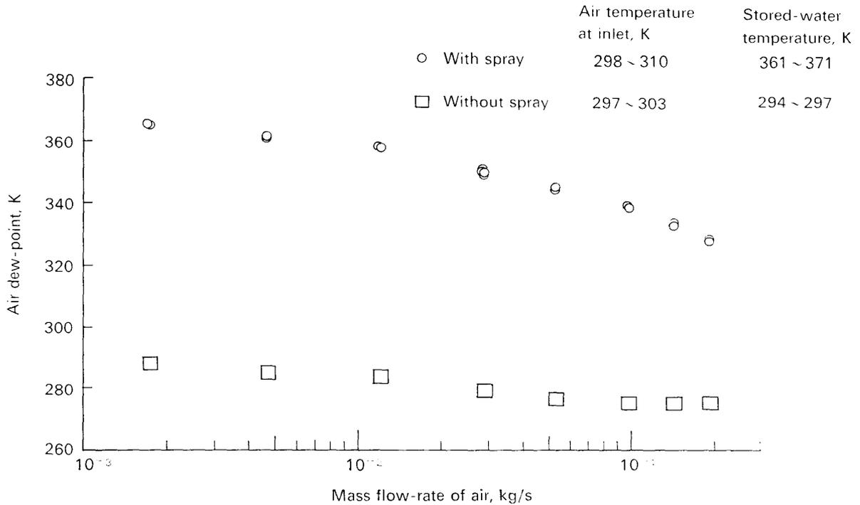
FIG. 8. Air dew-point at the outlet of the humidifying tower as a function of the mass flow-rate of the air entering the tower.
