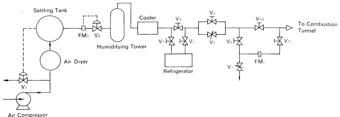
FIG. 1. Schematic flowchart of the system.
