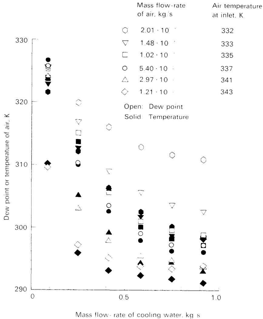
FIG. 10. Dew-point and temperature of the air at the outlet of the cooler, as a function of the mass flow-rate of the cooling water.
