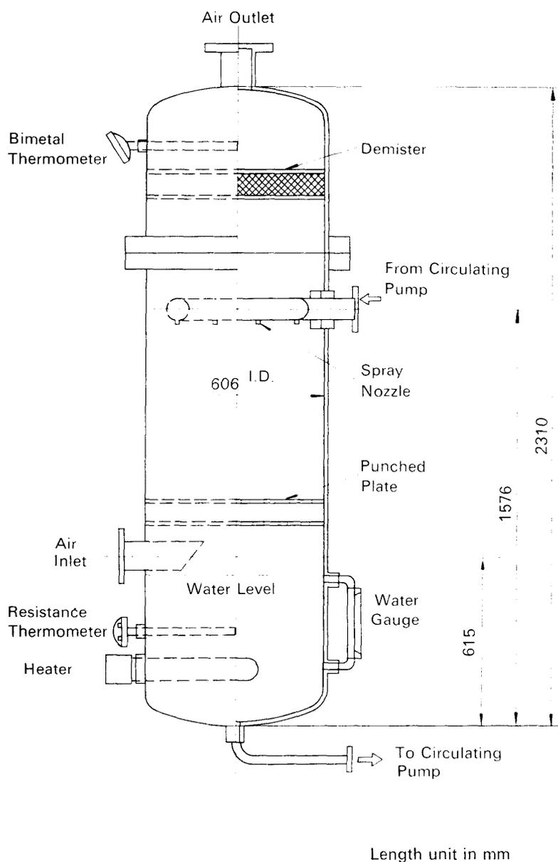
FIG. 4. Structure of the humidifying tower.
