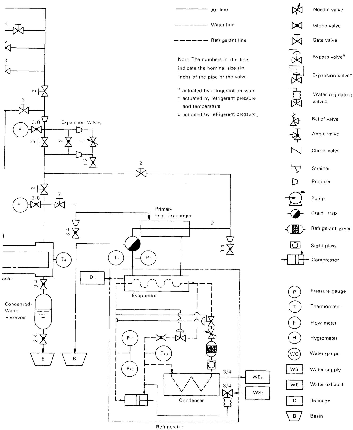
Schematic diagram of the main lines of the system.
