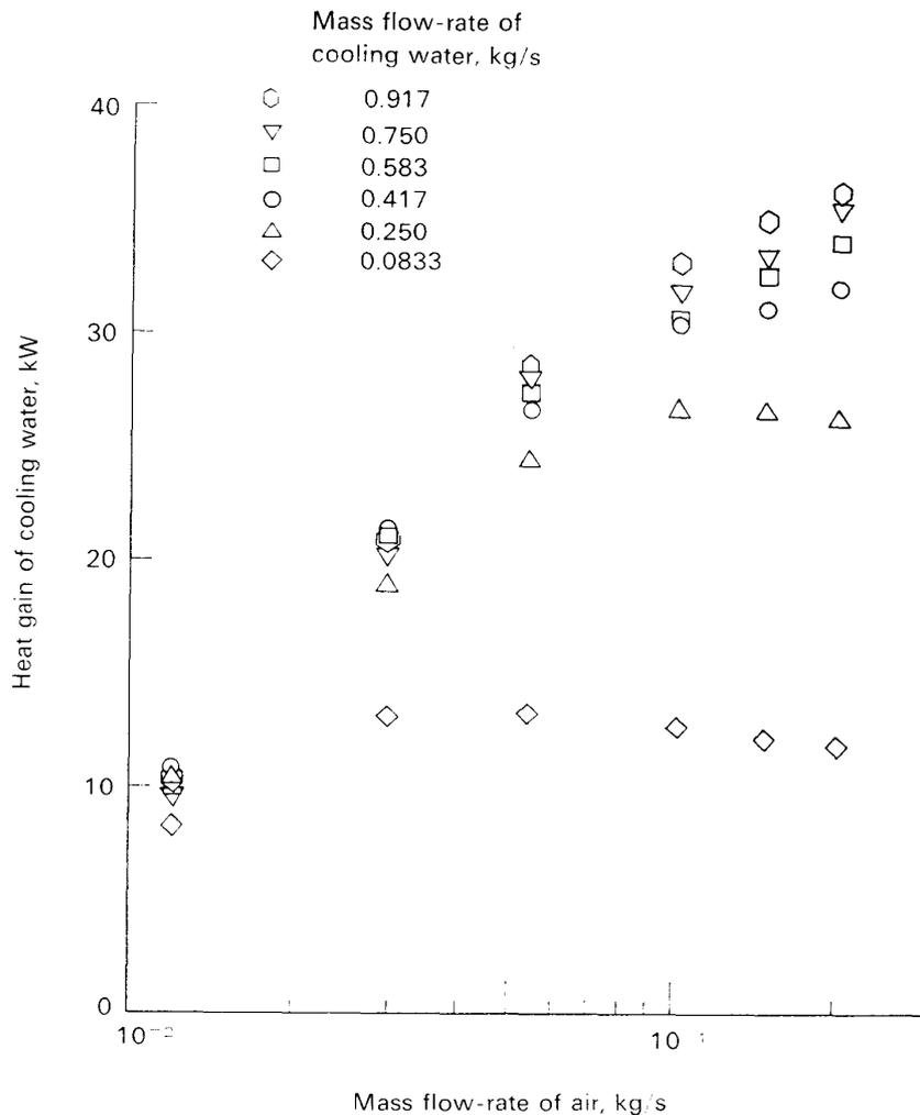
FIG. 13. Heat gain of the cooling water as a function of the mass flow-rate of the air; the temperature of the air at the cooler inlet ranges from 332 to 343 K.
