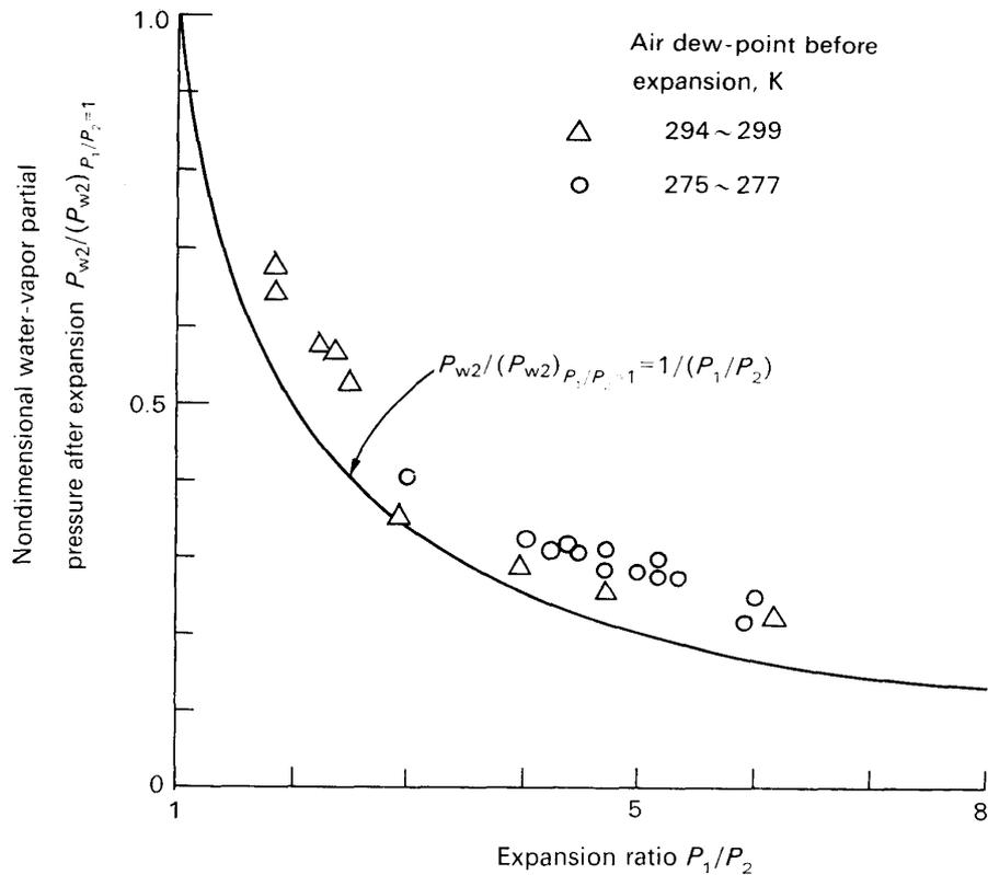
FIG. 7. Experimental results of the decrease in water-vapor partial pressure by expansion.
