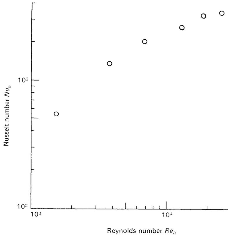
FIG. 14. Nusselt number for heat transfer (humid-air side) as a function of the Reynolds number of the humid-air flow.
