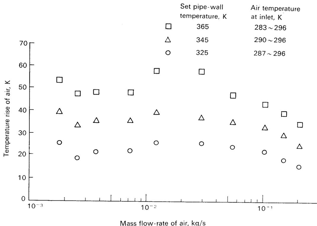
FIG. 11. Rise in the air temperature through the pipe-line heater as a function of the mass flow-rate of the air.
