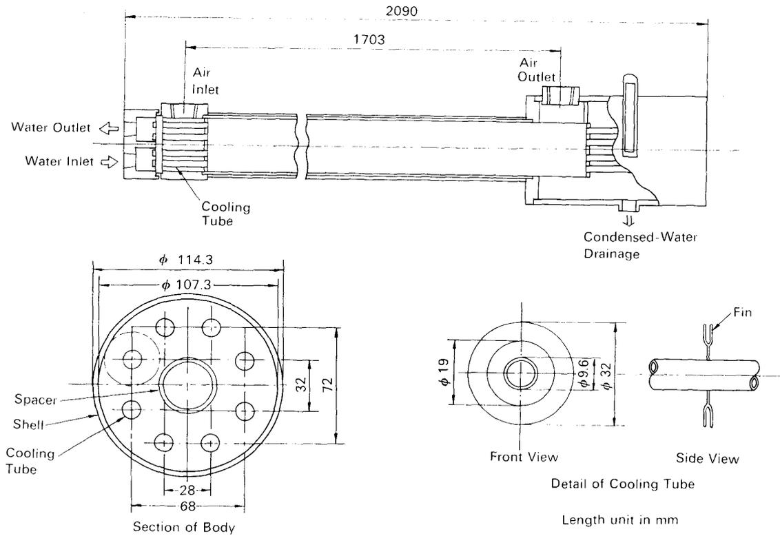
FIG. 5. Structure of the cooler.
