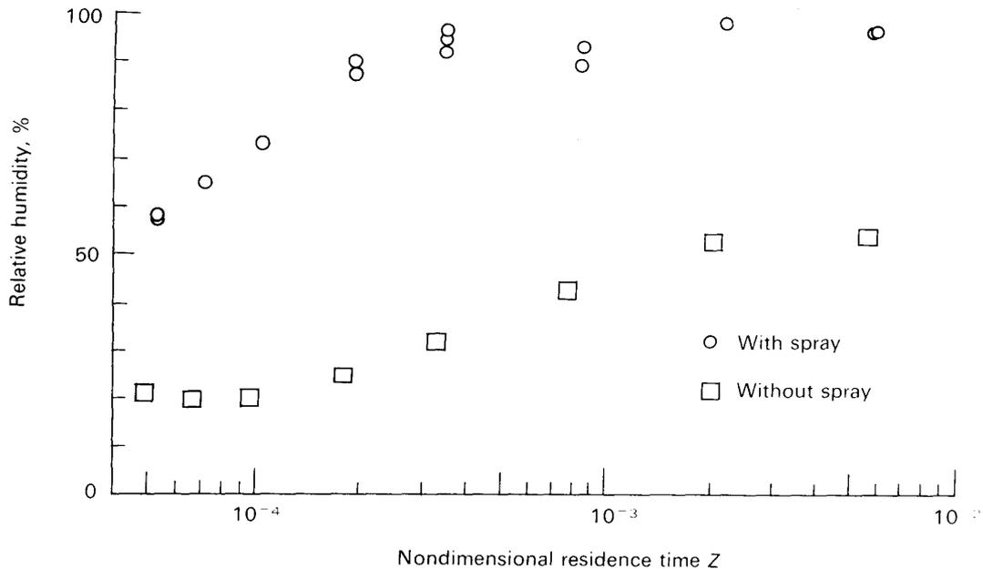
FIG. 9. Relative humidity of the air at the outlet of the humidifying tower as a function of the nondimensional residence time of the air.
