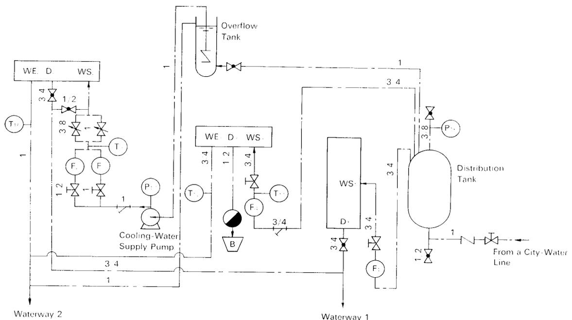
FIG. 3. Distribution diagram of the water-supplying and -draining lines of the system. (The meanings of the symbols are the same as in Fig. 2.)
