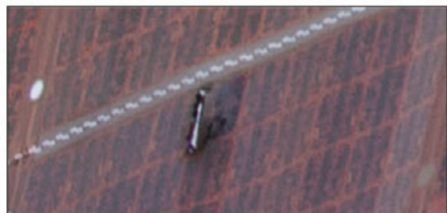
Figure 7. Another burned area in ISS Solar Array 3A (panel 42).
