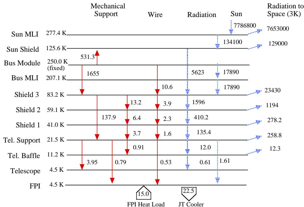
Fig. 3: Heat flow (unit: mW) diagram of the HII/L2 mission cooled by radiation and cryogenic coolers. Black arrows show the heat flow by conduction and shaded arrows show the heat flow by radiation. We assume a structure of the conceptual design (Figure 1)
