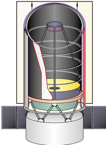
Fig. 1: Conceptual design of the HII/L2 mission with a 3.5 m primary mirror.
