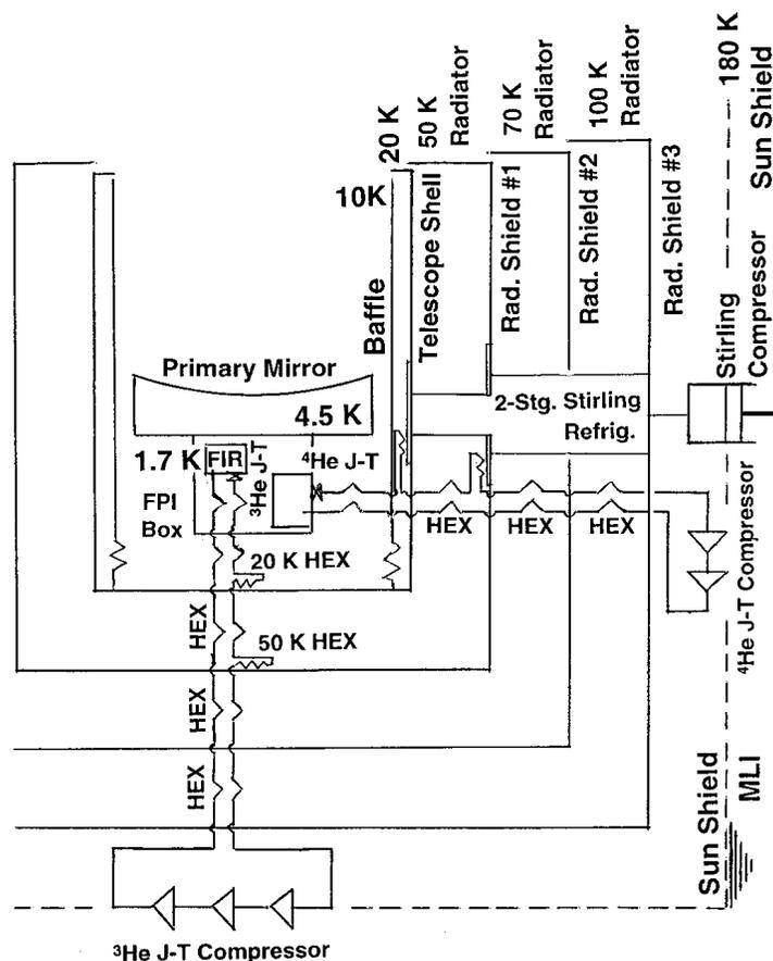
Fig. 2: Schematic drawing of the cryogenic system of the HII/L2 mission. The telescope is enshrouded with multi-layered radiators. One set of a JT cooler (with  $^4\text{He}$ ) and a two-stage Stirling cycle is used to cool the telescope and some of focal plane instruments to 4.5 K. Another set of a JT cooler (with  $^3\text{He}$ ) and a two-stage Stirling cycle is used to cool the far-infrared detectors to 1.7 K.
