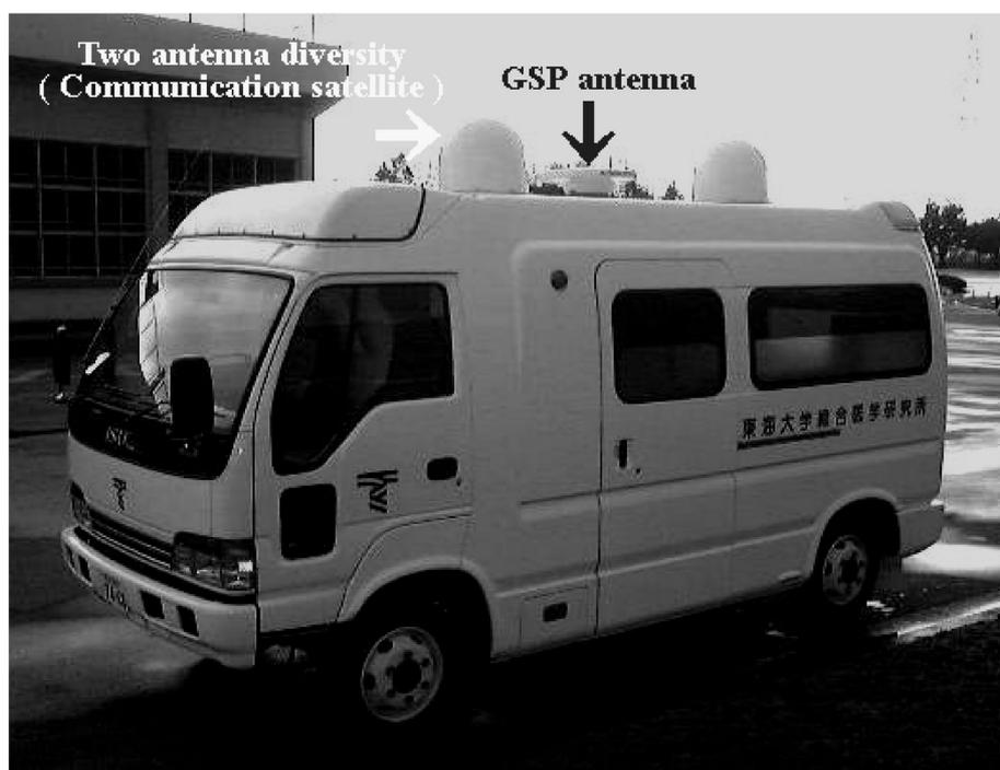
Fig. 1 GPS antenna for Continuous kinematic positioning
