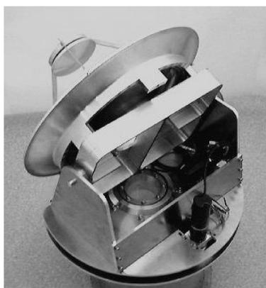
Fig. 3 On board antenna (40cm diameter Ku- Ka band)
