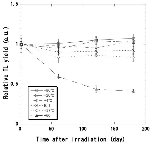
Fig. 6 Fading effect of  $Mg_2SiO_4$ :Tb irradiated by 10 mGy protons up to 6 months.
