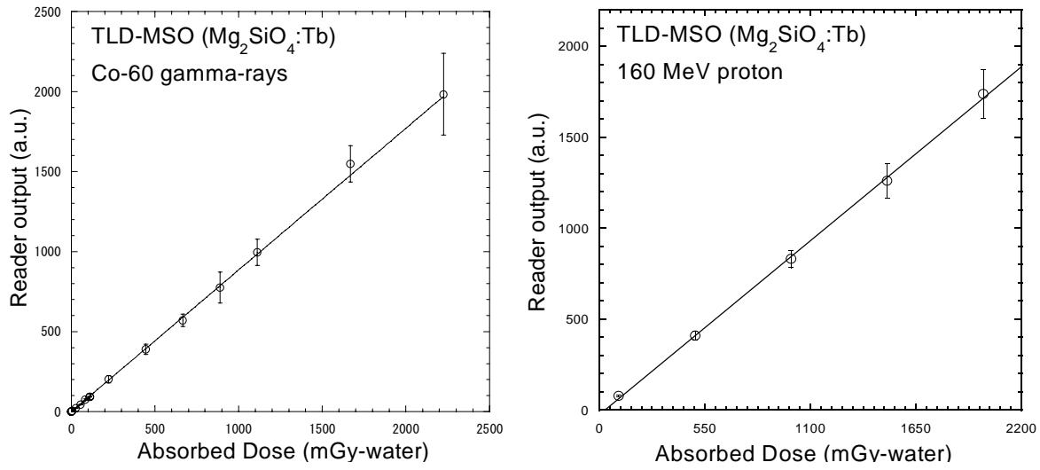
Fig. 5 Relative thermoluminescence yields of  $Mg_2SiO_4$ :Tb for gamma rays and 0.54 keV/ $\mu$ m protons as a function of an absorbed dose up to 2 Gy.
