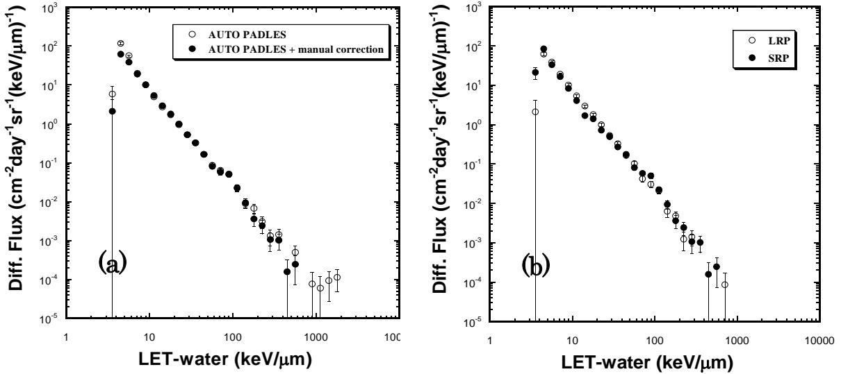
Fig. 7 LET distributions in the ISS Russian segment for 71 days. (a) Comparison of LET distributions measured by AutoPADLES without a manual correction for ellipse fitting of etch pits and that with the manual correction. (b) Comparison of LET distributions measured from a SRP sample and that from a LRP sample.
