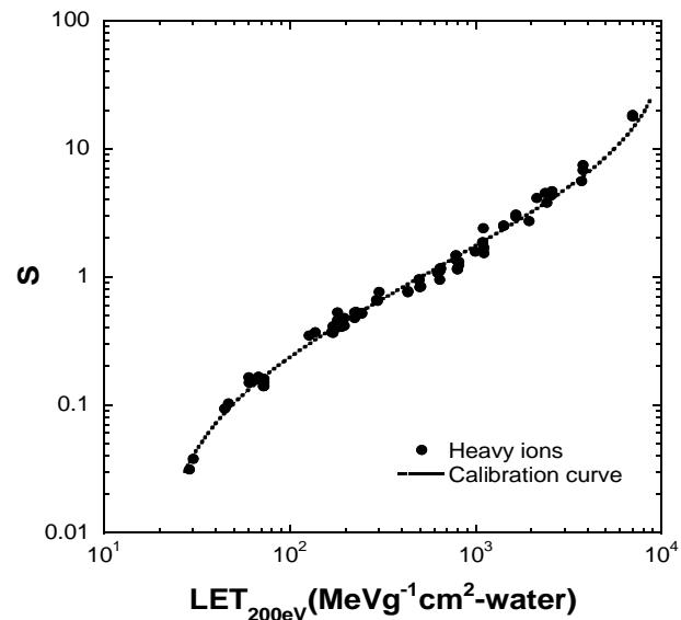
Fig. 4 Calibration curve for high-energy heavy ions of TD-1. The curve can be applied to both the 5.5 h and 13.5 h etched samples.
