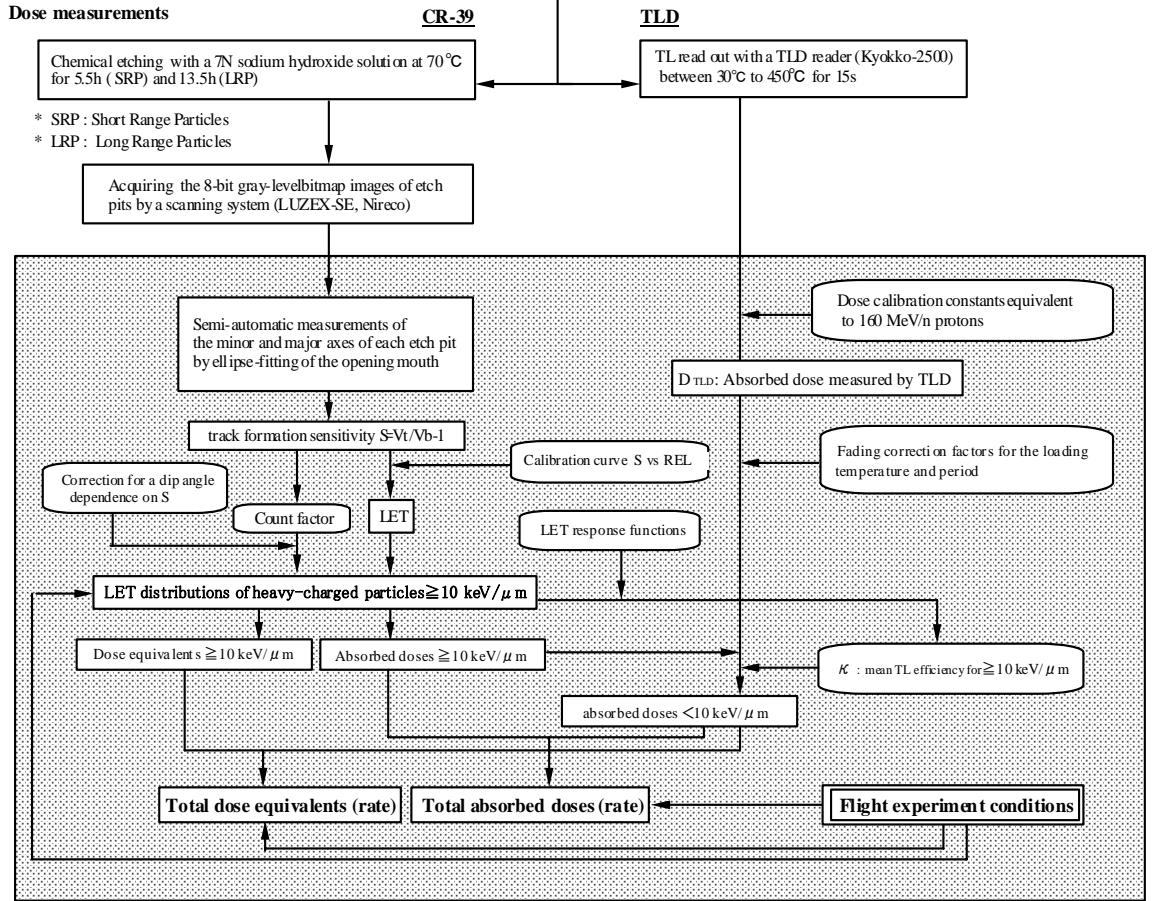
Fig. 2 Standard procedure of space radiation dosimetry by PADLES.
