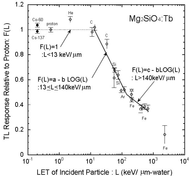
Fig. 1 TL response as a function of LET used in the PADLES system.
