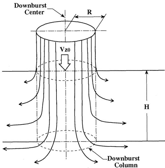
Fig.3 Structure of Windshear Model 1
