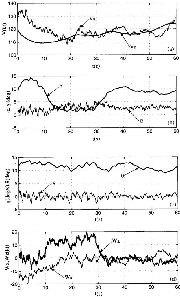
Fig.5 Simulation Result of Aircraft Take off in Windshear M 1
