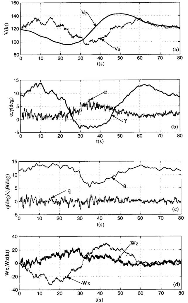
Fig.6 Simulation Result of Aircraft Take off in Windshear M 2
