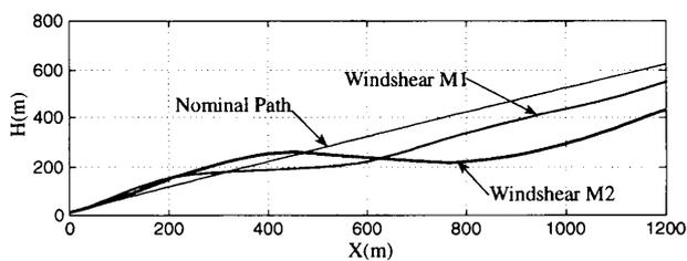
Fig.8 Flight Paths of Aircraft Take off in Windshear
