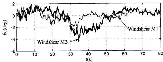
Fig.7 Elevator Control of Aircraft Take off in Windshear
