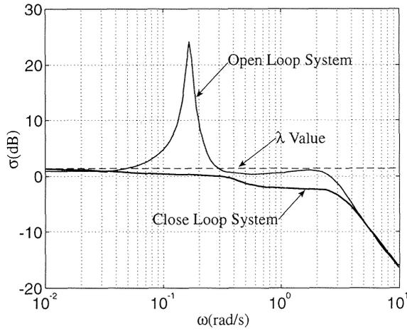
Fig.2 Maximum Singular Values of System
