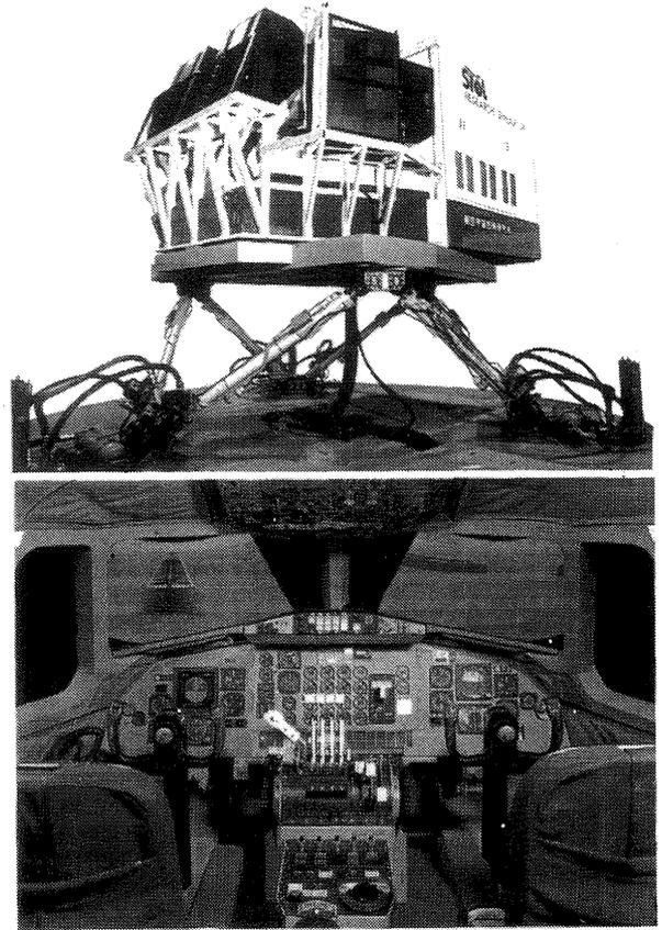
Fig.4 Six Degree-of-Freedom Flight Simulator
