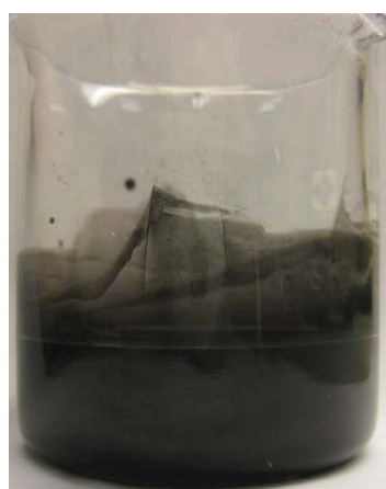
Un-bundled CNTs dispersed in solution
