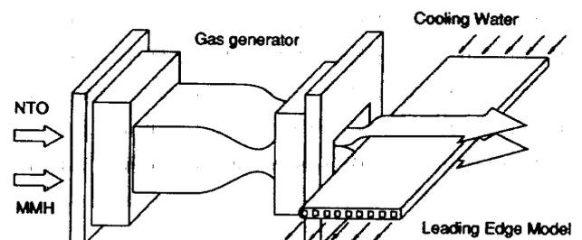
Figure 1. Schematic Representation of the Heating Test
