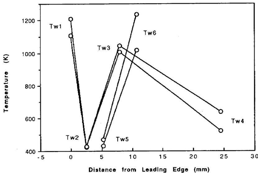
Figure 18. Measured Wall Temperature (Overexpansion test)
