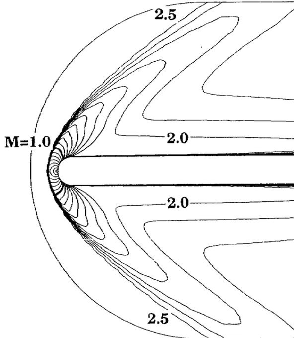
Figure 6. Mach Contour (Uniform flow)
