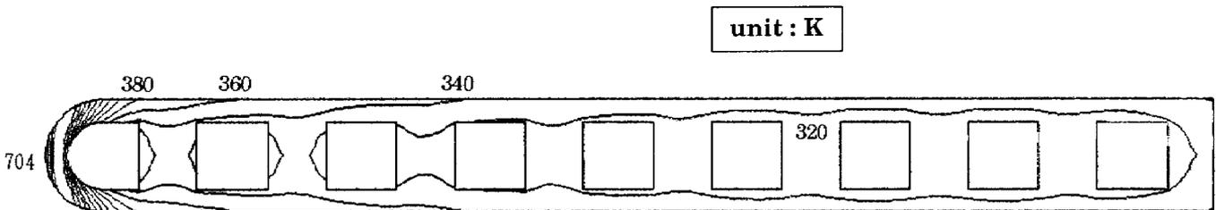
Figure 7. Temperature Contour (Uniform flow)
