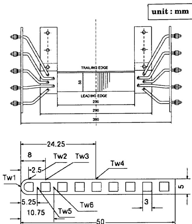
Figure 2. Crossflow Cooling Leading Edge Model
