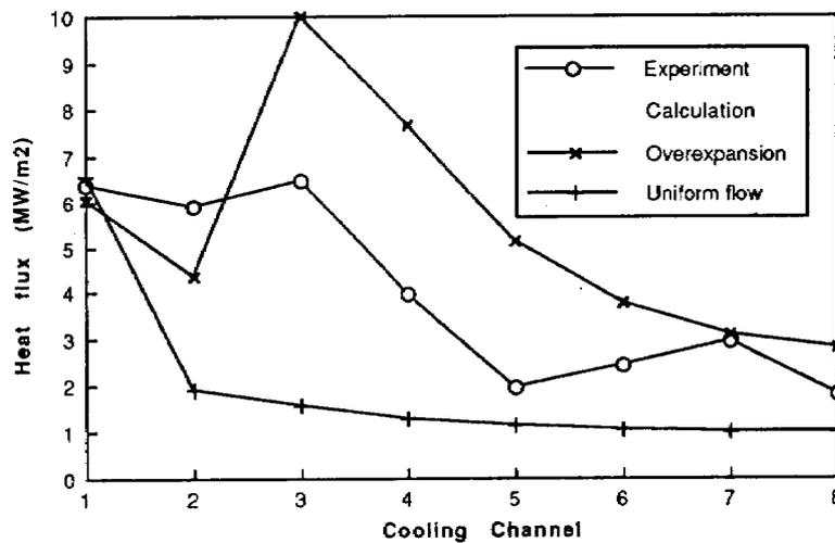
Figure 17. Mean Heat Flux Distribution (Overexpansion test)
