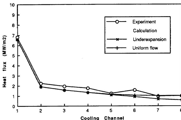
Figure 12. Mean Heat Flux Distribution (Underexpansion test)
