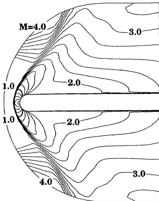
Figure 9. Mach Contour (Underexpansion)
