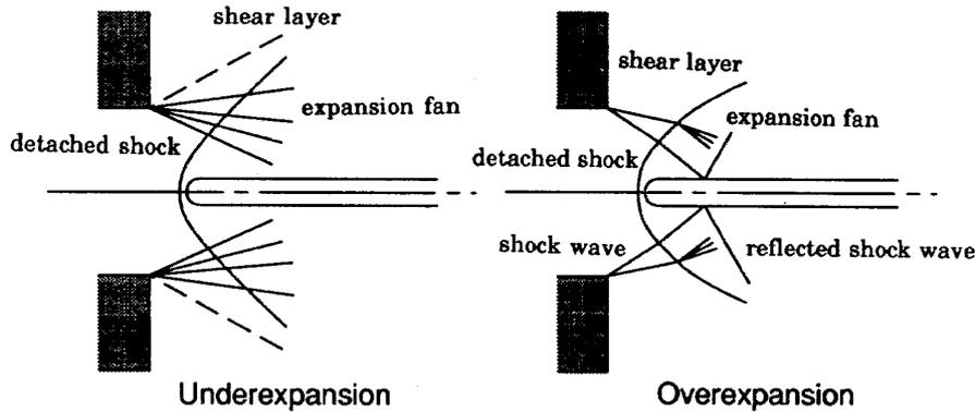
Figure 3. Interaction between the Test Panel and the Waves
