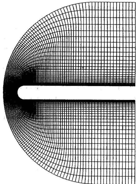
Figure 4. Numerical Grid around the Leading Edge Model
