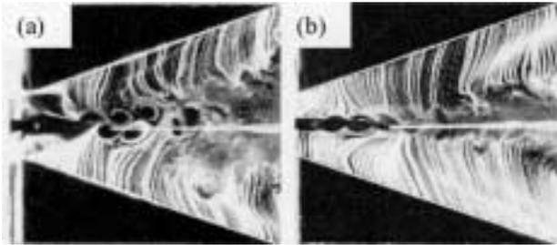
Fig. 3 Entrainment for (a) the antisymmetric excitation at  $u_f/U_0 = \pm 0.05$  and (b) the symmetric excitation at  $u_f/U_0 = \pm 0.10$ .
