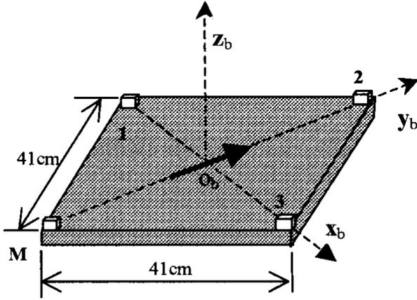
Fig. 2 TANS Vector's 4-antenna square configuration
