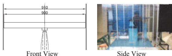
Fig.2 Quasi Two-Dimensional Flow Field
