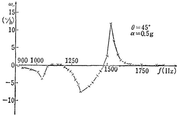
Fig. 10 Frequency characteristic of  $\omega_\alpha$  (Experimental result)
