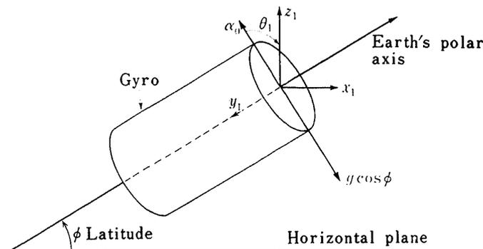
Fig. 4 Gyro output axis set parallel to earth's polar axis
