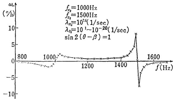
Fig. 13 Frequency characteristic of  $\omega_\alpha$  (simulation)
