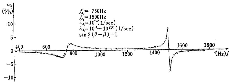
Fig. 12 Frequency characteristic of  $\omega_\alpha$  (simulation)
