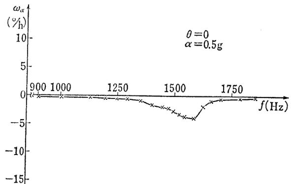
Fig. 9 Frequency characteristic of  $\omega_\alpha$  (Experimental result)
