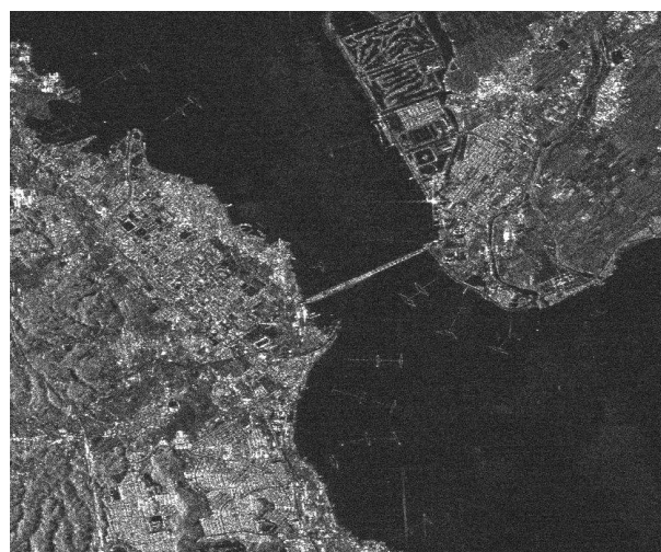
Figure 3. Full range resolution section of the PALSAR Kyoto image acquired on 21-Mar-2006. The slant range sampling corresponds to an approx. ground range sampling of 7.9 m, the azimuth pixel spacing (3-look) is 9.55 m.
