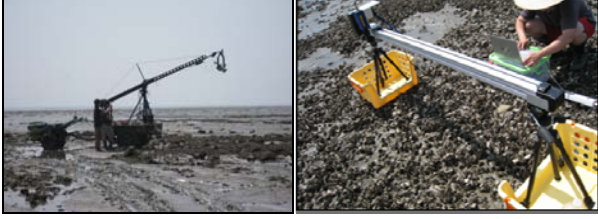
Fig. 2. In-situ measurements using a ground-based scatterometer system and laser surface profiler.
