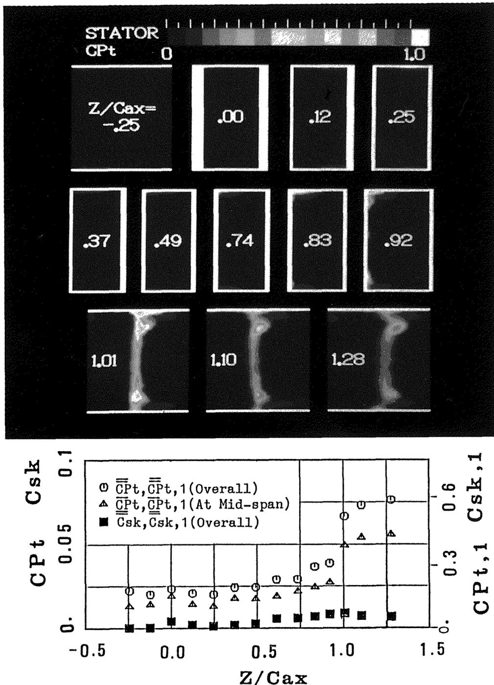
Fig. 7 Evolution of mass-averaged total pressure loss (straight stator cascade)
