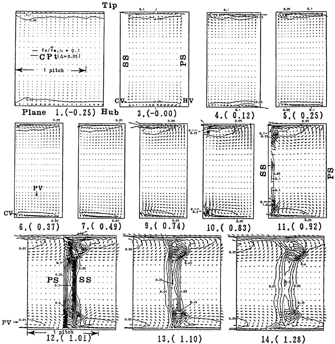
Fig. 3 Development of secondary flows and total pressure losses before, within, and after a straight stator cascade, S3 planes, ( $Z/C_{ax}$ )
