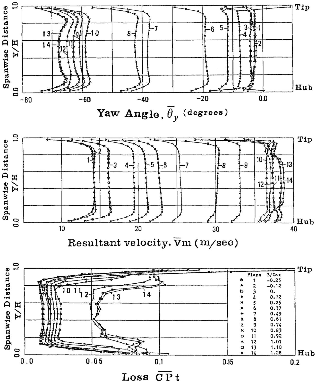
Fig. 6 Spanwise distribution of pitchwise-averaged yaw flow angle, resultant velocity, and total pressure loss coefficient
