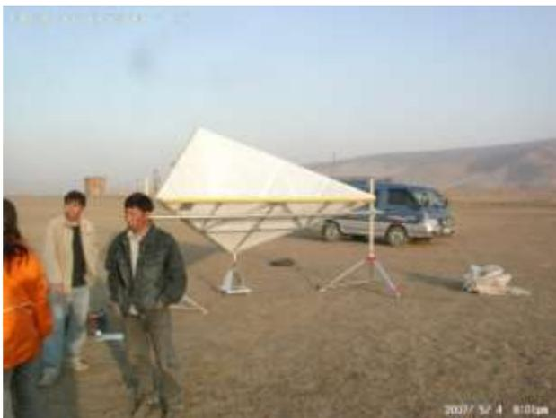
Fig. 2 2.5-m trihedral corner reflectors (CRs) deployed at the U-2 site (Ulaanbaatar) during field data collections.
