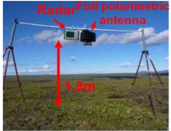
Fig. 7 Portable full polarimetric ground-based scatterometer.
