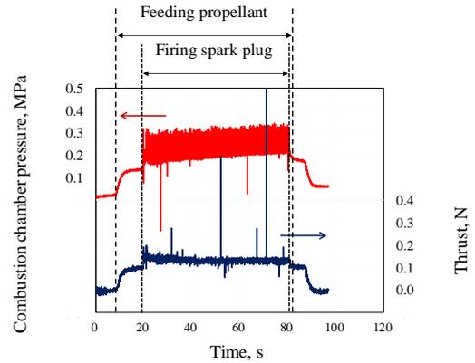
Fig. 6. Time history of combustion experiment: intermittent combustion
