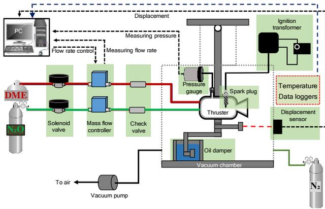
Fig. 4. Schematic diagram of the experiment apparatus
