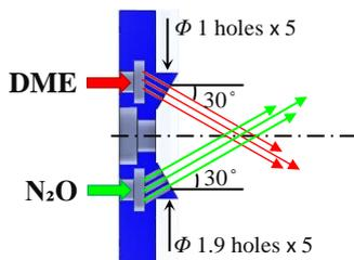
Fig. 2. Schematic of the impingement-type N<sub>2</sub>O/DME injector.
