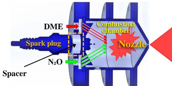
Fig. 1. Schematic of the prototype thruster
