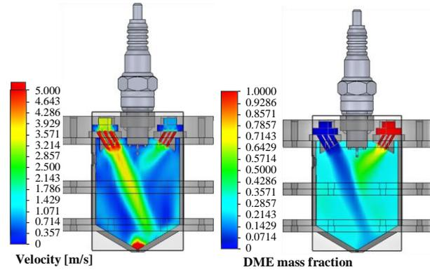
Fig. 3. Schematic of the flow simulation in the thrust chamber
