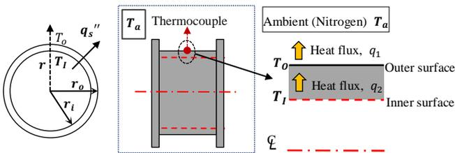
Fig. 9. Schematic of the upstream part of the thrust chamber
