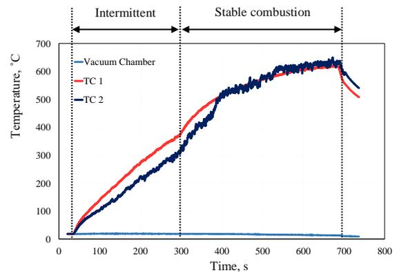
Fig. 8. Time histories of the outer surface temperature of the thrust chamber
