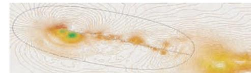
Fig. 25 Isobaric contours around the corrugated wing in the middle of upstroke.
