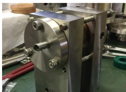
Figure 2 Stirred combustion type LOX vaporizer (Top view).
