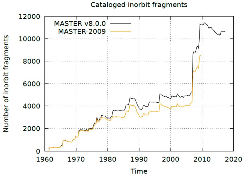
Various new TLE objects have been cataloged between 2009 and 2016, which can be traced back to fragmentation events that occurred in the early 1980s or even before.
