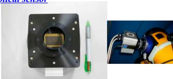
Large CMOS camera developed for LEO objects. The readout speed is 60 times faster than CCD.
