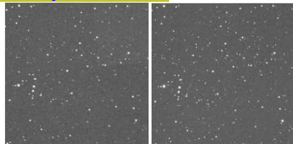
Difference between CCD frame(left) and CMOS frame(right) under the same condition
