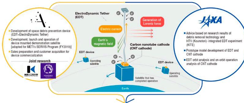
Extend conductive tether from EDT device mounted on microsatellite and de-orbit.
