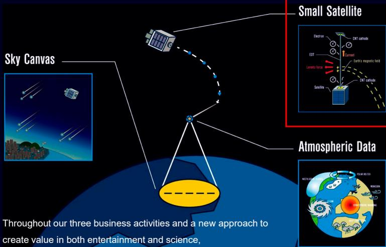
ALE, together with JAXA (Japan Aerospace Exploration Agency) has developed a space debris disposal device using Electrodynamic tether (EDT), enabling prompt deorbit of satellites after the completion of their mission.
