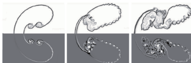
Deformation of helium bubble due to shock wave passage in air
