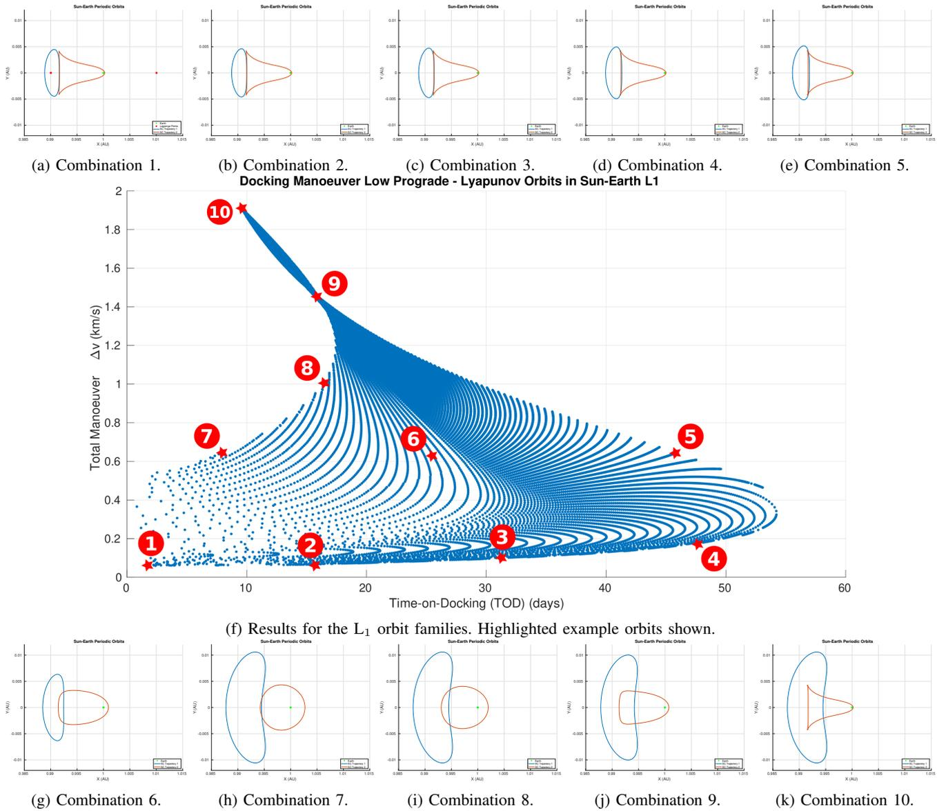
Fig. 10: SODI Manoeuvre  $\Delta v$  (insertion to and exit from Lyapunov Orbit) vs TOD (Time-on-Docking, time spent in the Lyapunov Orbit between the two maneuvers). Highlighted are some selected example orbits.
