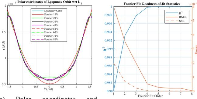
(a) Polar coordinates and Fourier (1-8 orders) Fits for a parametrized Lyapunov Orbit with respect to the  $L$  point. (b) Fourier Fit Goodness-of-fit Statistics with respect to the fit order. Statistics for the orbit in Fig. 7a
