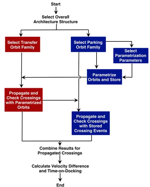
Fig. 5: Flow Chart summary of the Single Orbit Dual Insertion (SODI) Finding Algorithm.
