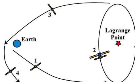
Fig. 1: DS-OTV architecture. 1) The spacecraft transfers to the DS-OTV parking orbit. 2) It docks with the DS-OTV to re-fuel. 3) It undocks and leaves the parking orbit. 4) After an Earth Swing-by, the spacecraft starts its journey to the objective.
