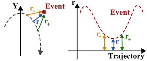
Fig. 8: Crossing event check (left) and event distance minimum search graph (right).
