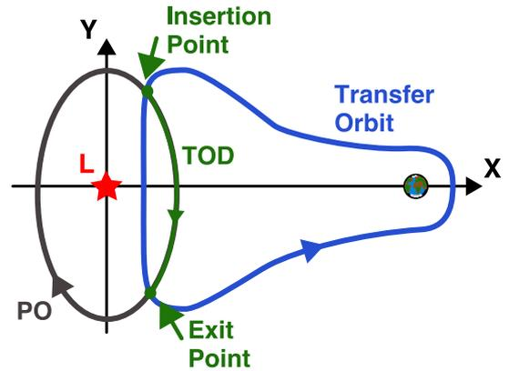
Fig. 9: A Single Orbit Dual Insertion maneuver, with the Time-on-Docking (TOD) marked.
