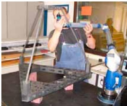
Fig. 3.2-2 Integrated Support Structure and Its 3D Measurement
