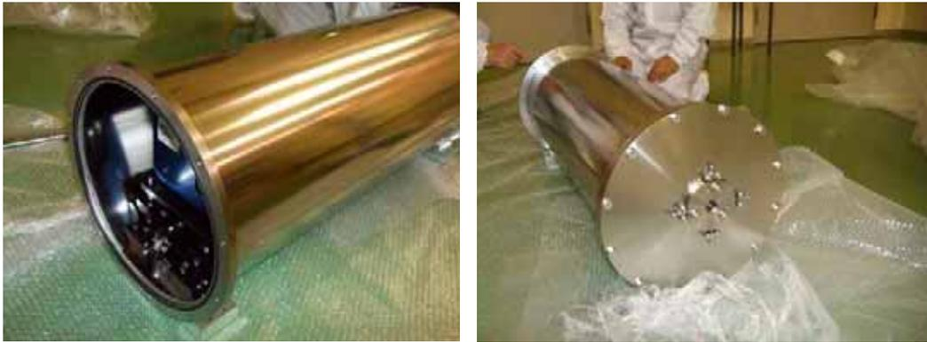
Fig. 3.2-6 Pressure Vessel for the Interferometer
