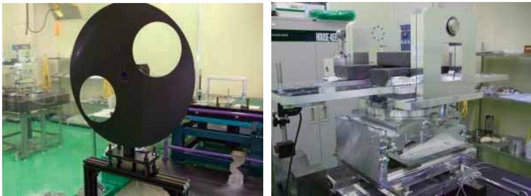
Fig. 3.2-5 Rotation Mask for Stitching Simulation (left) and 5-axis Precision Stage (right)
