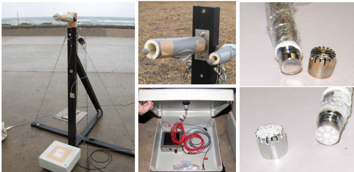
Fig.3-1. A microphone stand and a microphone box on the ground (left).
