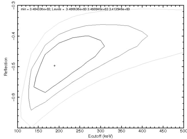
Fig. 2. Confidence contours at 68, 90, and 99% level for the reflection albedo versus the power law energy cutoff.
