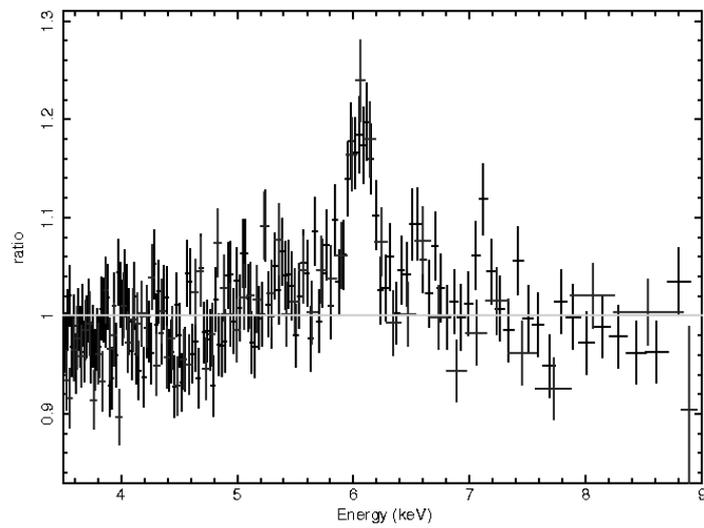
Fig. 3. Zoom-in of the Fe K line region in the Suzaku XIS spectrum of 3C 382. Blue: XIS1, Black: XIS0+3. The narrow core of the Fe  $K\alpha$  line, plus two additional emission lines at 6.5 and 7.5 keV can be easily seen.
