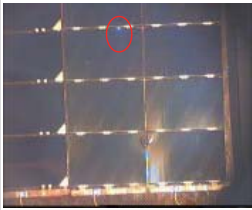
Minor Arcs shown at different locations between inter connectors.
