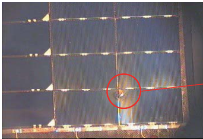
Minor Arcs shown at different locations between inter connectors.
