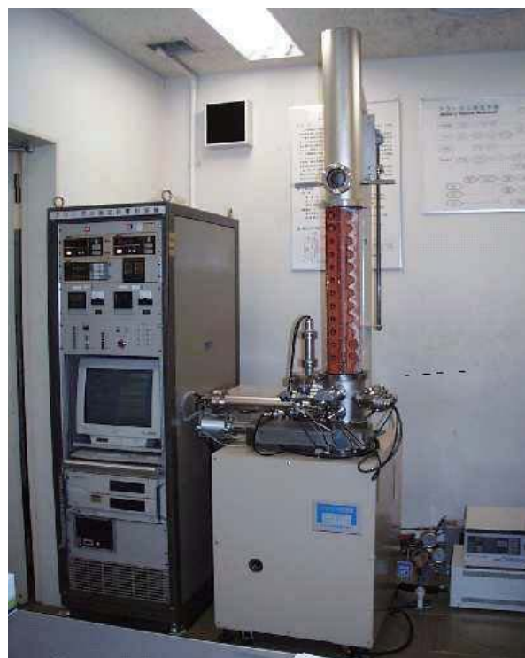
Fig. 2-4 Outgassing measuring system
