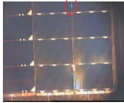
Minor Arcs shown at different locations between inter connectors.
