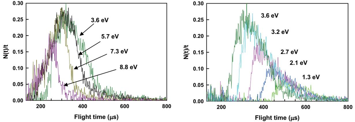
**Figure 3** Time-of-flight spectra of atomic oxygen beam ( $m/e=16$ ) sliced by the high-speed chopper wheel. For better view of the each TOF spectrum, left and right panels show the TOF spectra in which slow-part and fast-part of the beam pulses are blocked by the chopper wheel. The same TOF spectrum ( $E_{coll}=3.6$  eV) is shown in both panels for comparison purpose.
