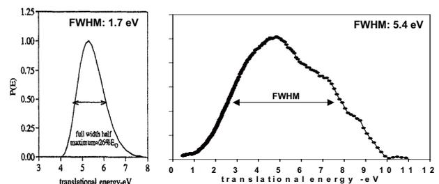
**Figure 2.** The energy distribution of atomic oxygen in low earth orbit space environment (left panel) and in laboratory simulated by a laser detonation source (right panel). Full-width at half-maximum (FWHM) is 1.7 eV and 5.4 eV for low earth orbit and for laboratory, respectively.
