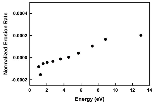
**Figure 5** Normalized erosion rate of polyimide as a function of collision energy of atomic oxygen. Difference in atomic oxygen fluxes in the sliced beam was compensated with dividing by the area of TOF spectrum of the each beam.
