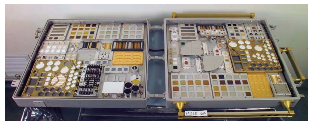
Fig. 4. Materials International Space Station Experiments (MISSE-6) pallet.
