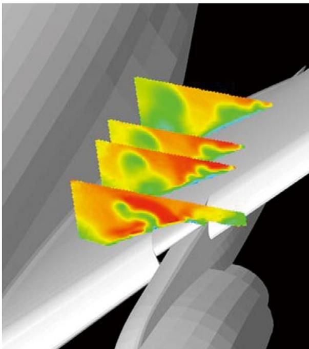
Fig.4 Vortices on wing behind nacelle
