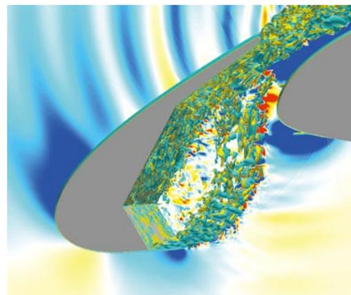
Fig.4 Analysis of noise around leading edge of high-lift slats
