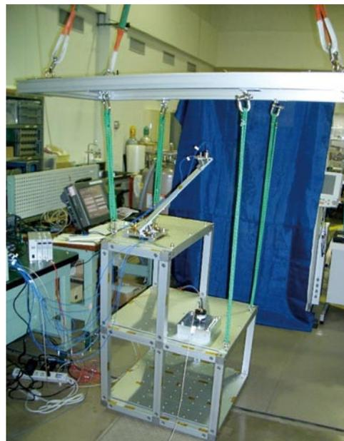
Fig.1 Laboratory-Scale Specimen with a Reaction Wheel for Microvibration Transmission Measurement
