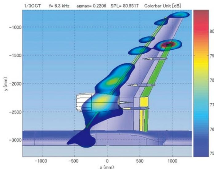
Fig.3 Contour of noise emitted from various positions on a wing
