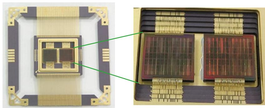
Fig.3 Stacked structure of 36 Mbit synchronous burst SRAM (Top view)
