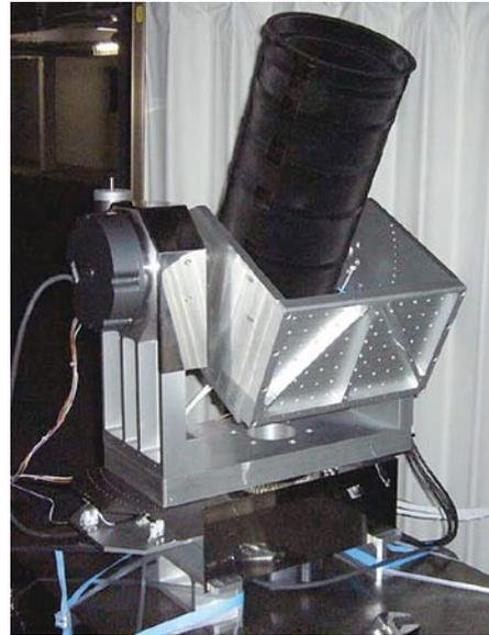
Fig. 1 High-performance autonomous star tracker research model real sky test
