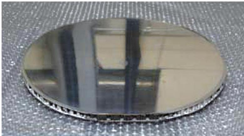
Fig.3 High Precision Mirror of CFRP / CFRP Honeycomb Core Sandwich Structure
