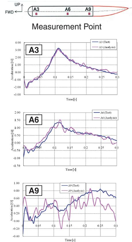
Fig.7 Accelerations in a horizontal-impact test case
