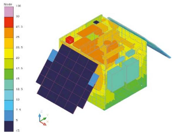
Fig.5 Thermal design analyses of SDS-1
