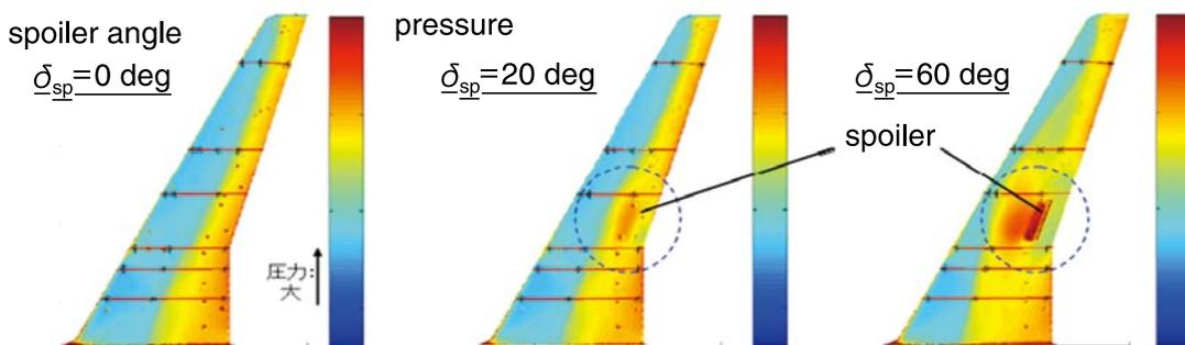
Fig.2 Surface pressures on wings with different spoiler angles
