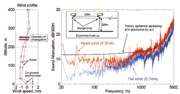
Fig.5 (top) Overview of the acoustic measurement using balloons. (bottom) Propagation effect of vertical wind profile.
