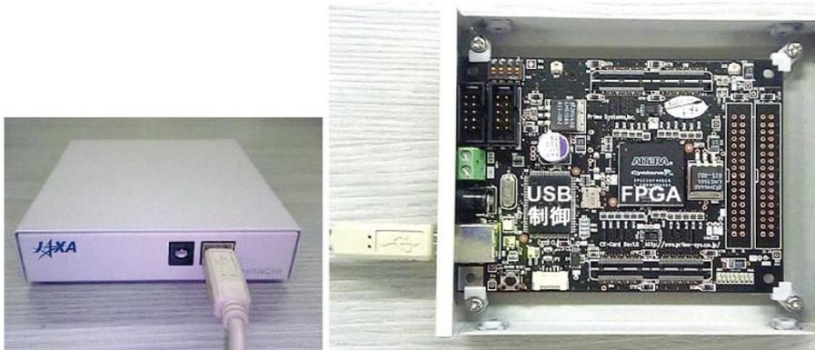
Fig.4 Prototype of error control circuit
