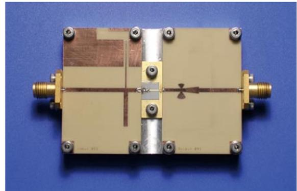
Fig.4 Trial model of an F class amplifier in the 5.8 GHz band that is used as the transmitting antenna for M-SSPS.
