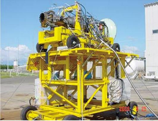
Fig.5 Low-noise nozzle noise test
