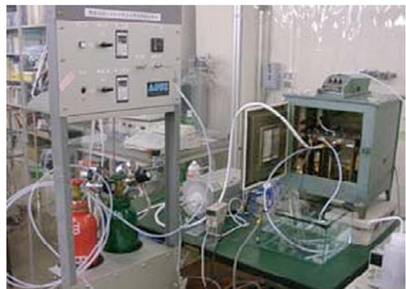
Fig.7 Air revitalization system with Sabatier reactor and water electrolysis for microgravity conditions
