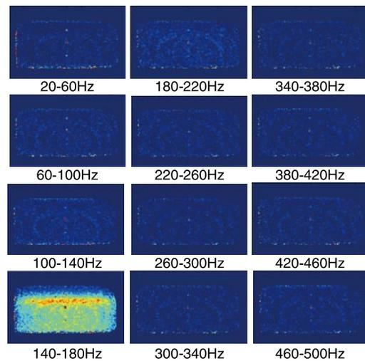
Fig.2(b) Unsteady pressure distribution over a cylinder in various frequency ranges.
