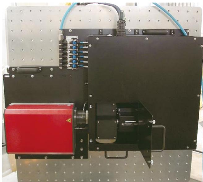
*Fig.3 High-power laser-diode heating system with bi-axial galvano scanner*
