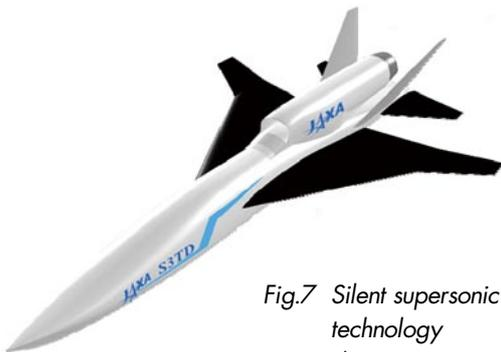
Fig.7 Silent supersonic technology demonstrator
