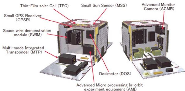
Fig.3 Mission equipment of SDS-1
