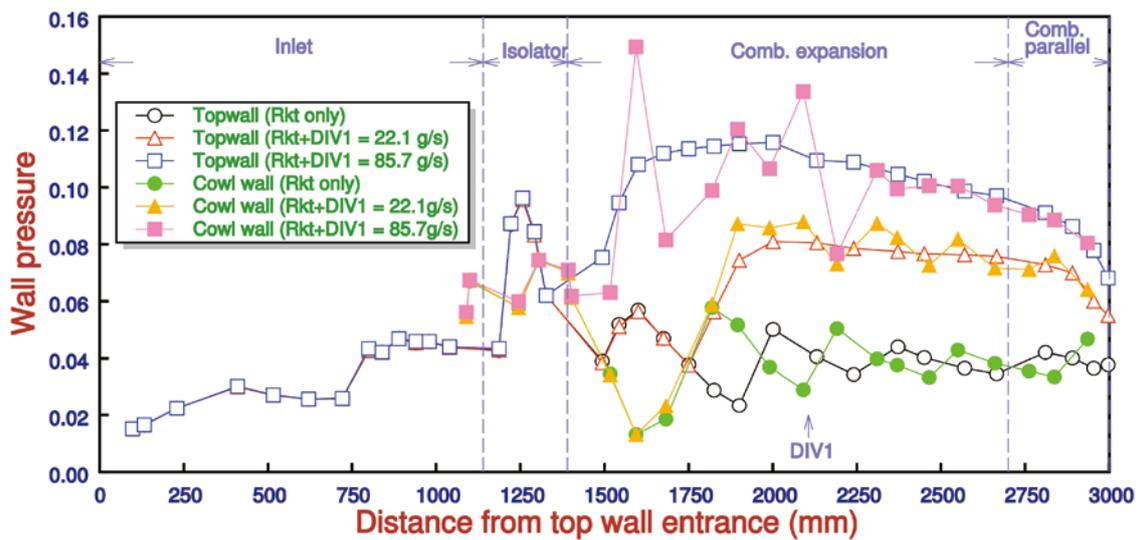
Fig.3 Wall pressure distribution in ramjet mode
