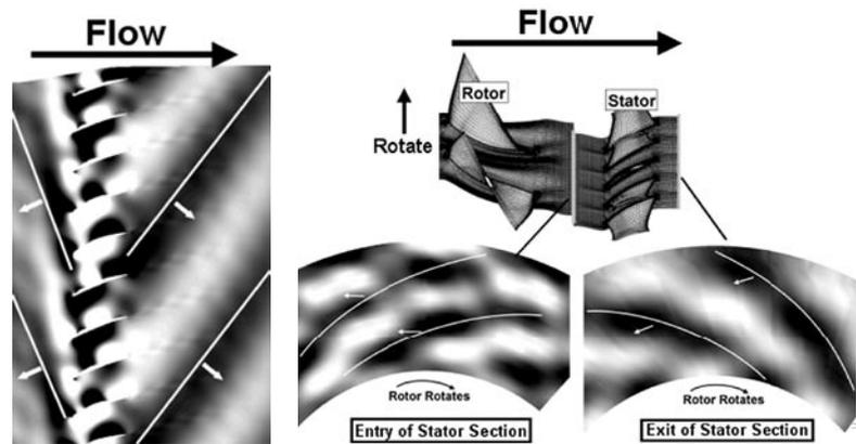
Fig.2 Pressure fluctuation contours around stator vanes showing mid-height, entry and exit.
