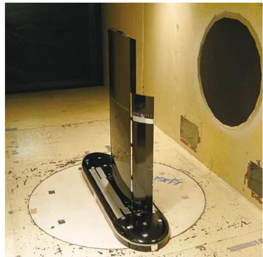
Fig.2 Model for high-lift device noise measurement (OTOMO)
