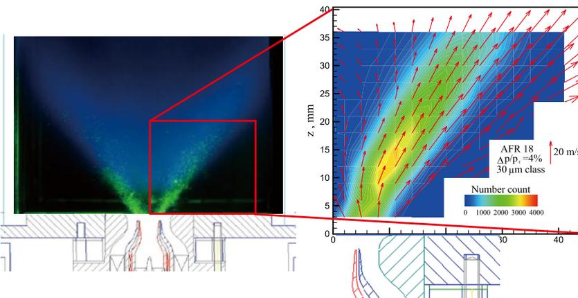
Fig.7 Number of droplets and velocity distribution of droplets from air-blast fuel nozzle (by stereo interferometric laser imaging technique)
