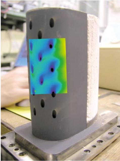
Fig.8 Cooling structure test piece and temperature distribution (montage)
