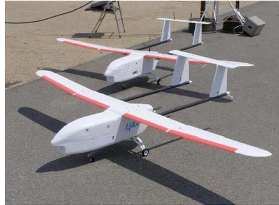
Fig.3 Electric Powered Fixed-wing UAV (2m span)
