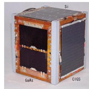
Fig.5 The micro-satellite "Cubesat XI-V" developed by the University of Tokyo. One mission of the satellite is to demonstrate the super-high radiation resistance of a CuInGaSe<sub>2</sub> solar cell.
