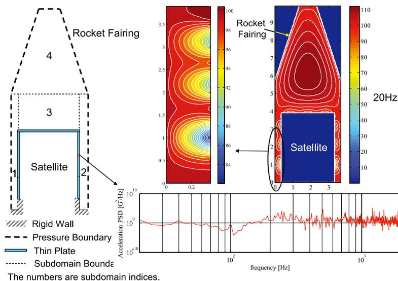
Fig. 1 Acoustic environment within the rocket fairing and vibration of the satellite surface.
