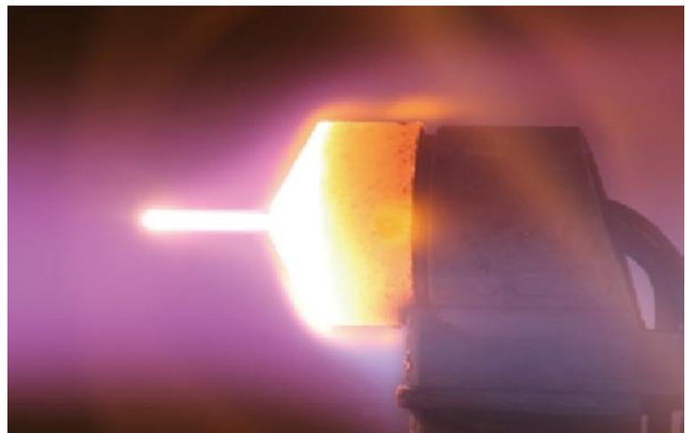
Fig.4(b) Heating test of a graphite test piece in a plasma wind tunnel with nitrogen as the working gas.
