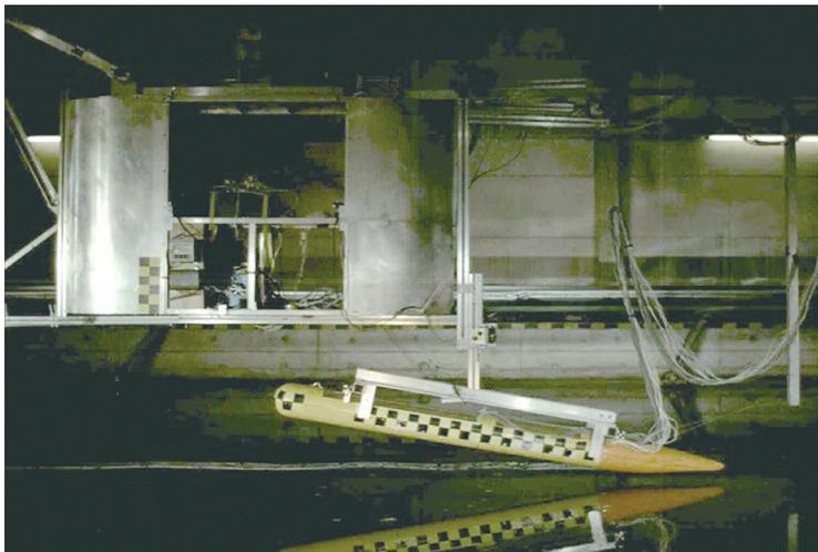
Fig.5 Horizontal water impact test model set-up
