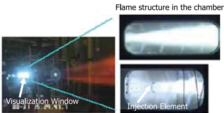
Fig.4 Propellant injection element test
