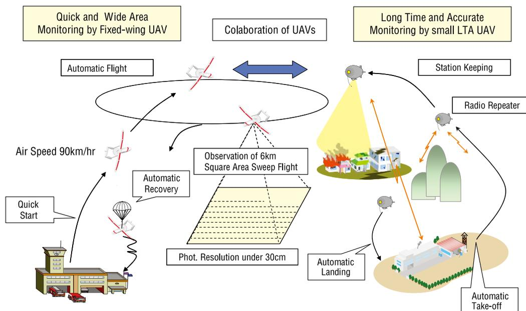
Fig. 1 Disaster Monitoring UAV System by Coordinated Fixed-wing UAV and LTA UAV
