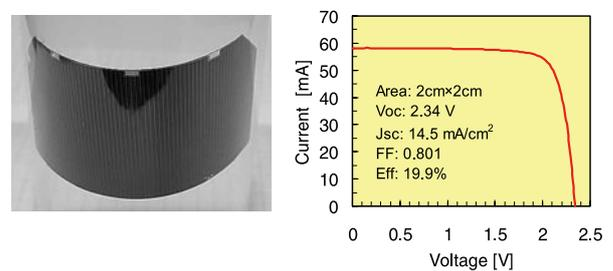
Fig.4 A prototype InGaP/GaAs dual-junction thin film solar cell and its current-voltage output characteristics.
