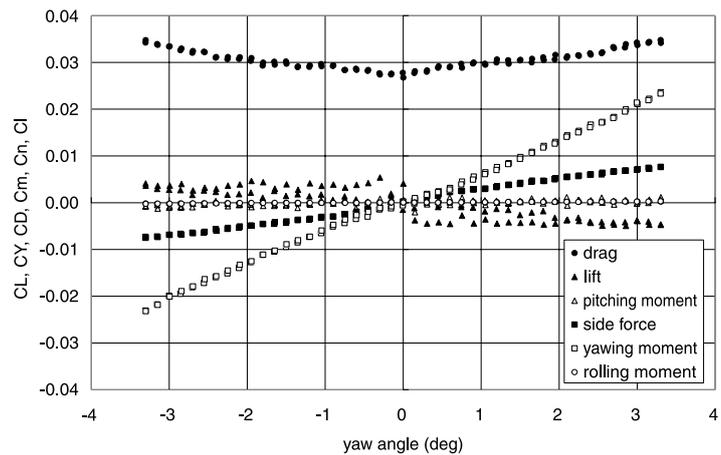
Fig.1(a) Measured all static aerodynamic coefficients of a winged model during its yaw angle change at 30 m/s in flow speed.
