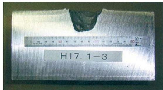
Fig.3 Collision of 1g bullet with thick aluminum plate at 7 km/s (cross section)
