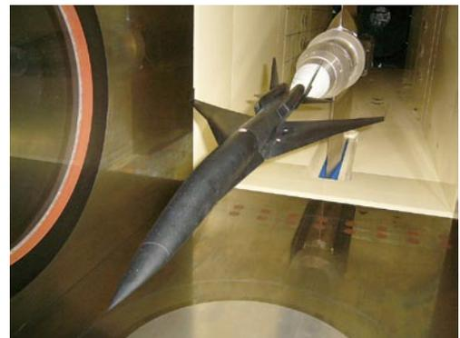
Fig.3 Supersonic wind tunnel test of quiet small supersonic transport concept
