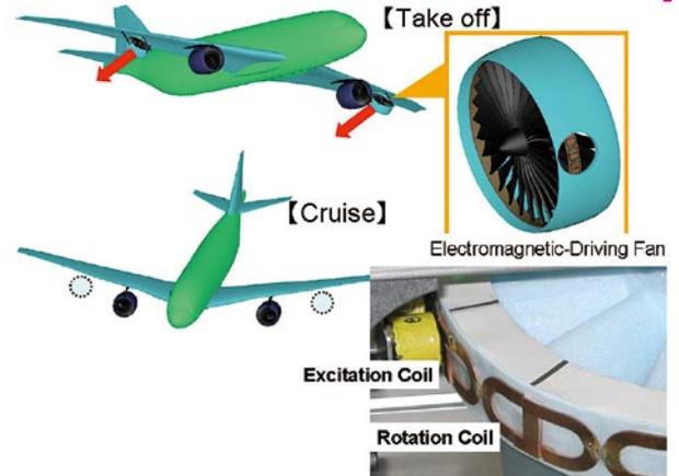
Fig.4 Conceptual diagram of an electric fan engine system and proof-of-principle model
