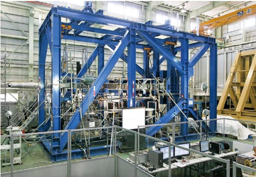
Fig.4 Full-scale test of VaRTM wing structure
