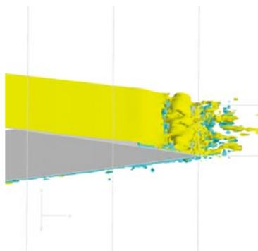
Fig.3(c) Vorticity distribution around the trailing edge on the pressure side
