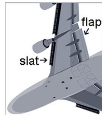
Fig. 1 Example of typical high-lift device
