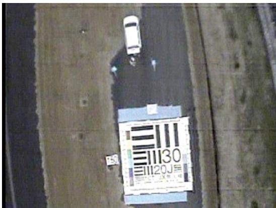
Fig.4 Test pattern on the ground for image resolution evaluation
