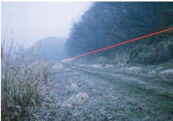
Fig.3 This image is preliminary experiment of laser energy transmission in Kakuda Space Center. Now a higher power experiment of about 0.8 kW is being carried out at this facility.
