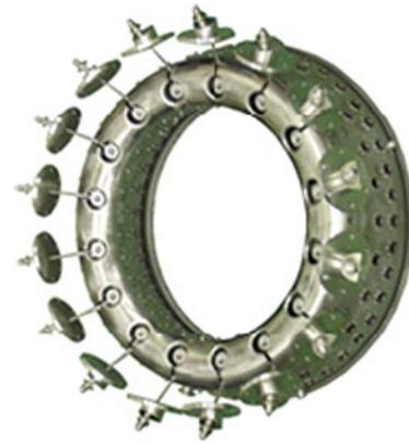
Fig.4 Low NOx combustor for small engine
