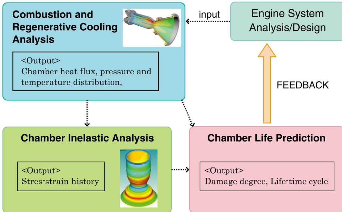
Fig.6 Combustion chamber coupled analyses
