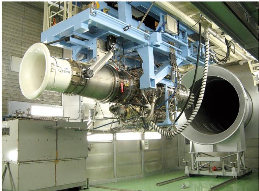
Fig. 1 ESPR engine installed in engine test cell
