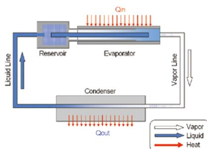
(a) Principle of loop heat pipe
