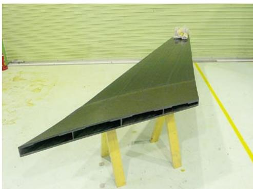
Fig.4 Composite material structure wing demonstrator
