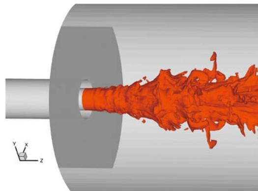
Fig.4 Instantaneous flame structure in the vicinity of a super-critical and cryogenic co-axial injector.
