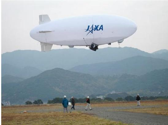
Fig.2 Small Unmanned Airship (14m long)
