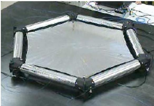
Fig.5 Trial model of an inflatable expandable structure that is a candidate for the large structure of an SSPS.
