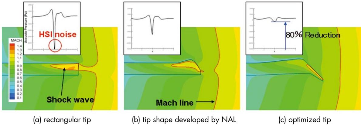
Fig.2 Mach contour and sound wave form of conventional and improved blade tip shapes.
