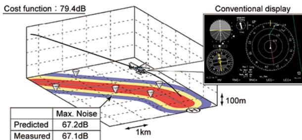
Fig. 1 Optimal noise abatement system. The results show a 4dB reduction in the average of the noise levels at 5 observation points.
