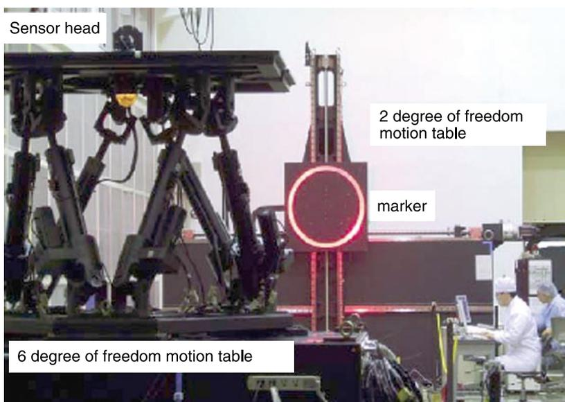
Fig.3 Test of the image navigation sensor
