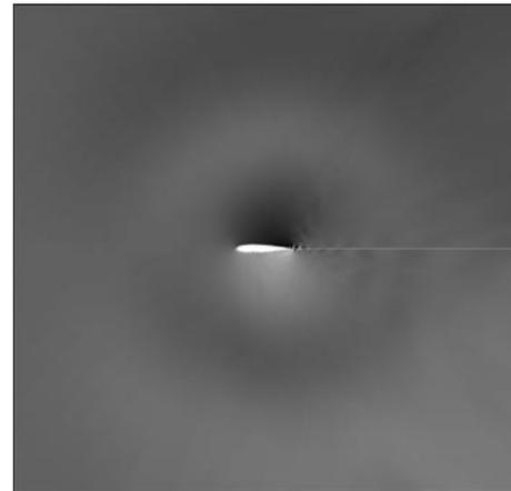
Fig.3(a) Instantaneous pressure fluctuation around NACA0015 wing profile at mid-span
