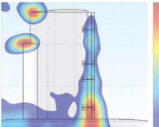
Fig.3 Indication of noise generation positions by source location.
