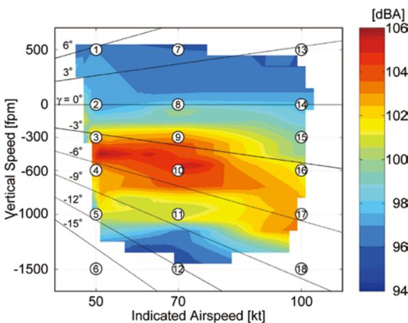
Fig.4 Noise levels obtained by the onboard external microphone. The loudest noise was observed in the normal approach flight condition (airspeed of 70 kt and descent rate of 600 fpm).
