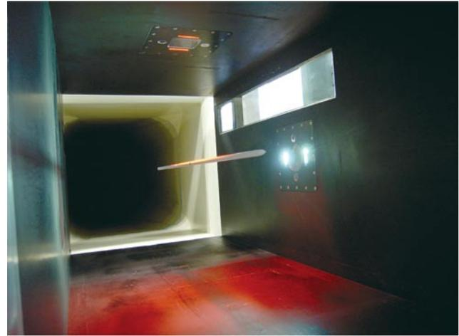
Fig.1(c) A magnetically suspended cylindrical model (10 mm diameter, 750 mm long) in the JAXA 60 cm magnetic suspension and balance system.
