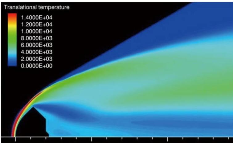
Fig.4(a) Distribution of translational temperature around HAYABUSA-type capsule in continuum flow ( $V = 11.4$  km/s, alt. = 64 km).
