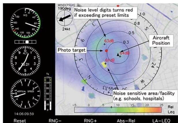
Fig. 2 Onboard display of cumulative and instantaneous noise. Pilots can easily avoid causing excess noise where quiet is required, even in unfamiliar areas.
