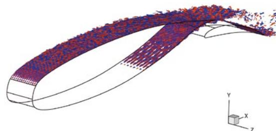
Fig.3(d) Vorticity distribution around an NLR7301 wing with flap
