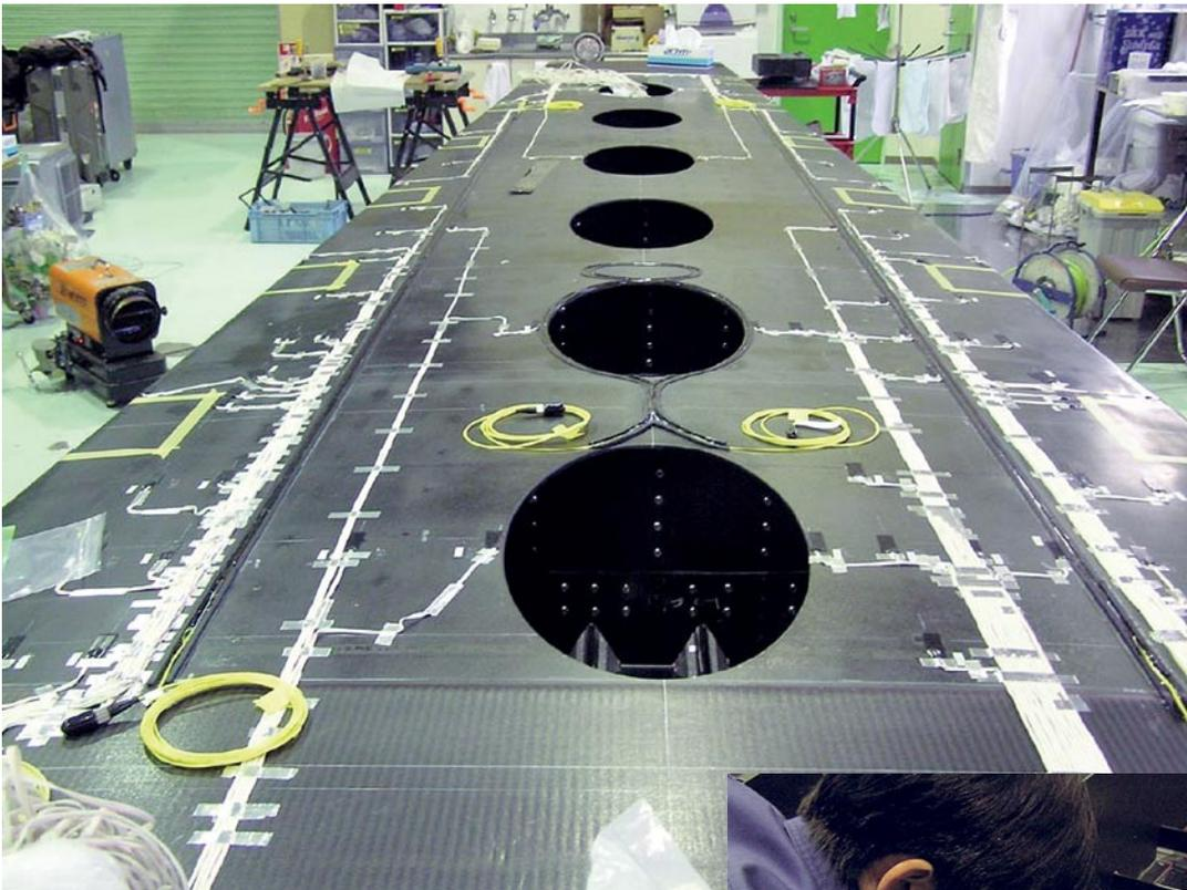
Fig.2 Fiber optic sensor system applied to full scale composite wing structure testing
