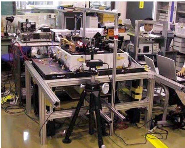
Fig.4 GOSAT TANSO-FTS BBM Microvibration Test Setup
