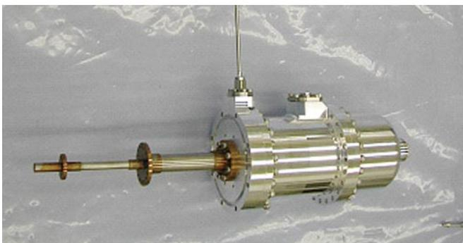
Fig.2 Modified coldhead of 20 K-class two-stage Stirling cooler
