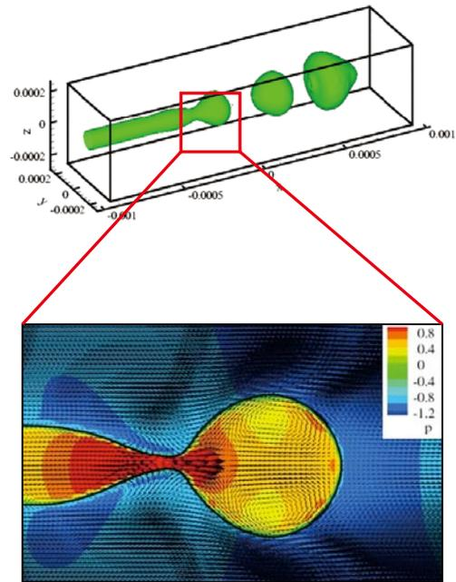
Fig.3 Droplet break-up by a propagative capillary wave.
