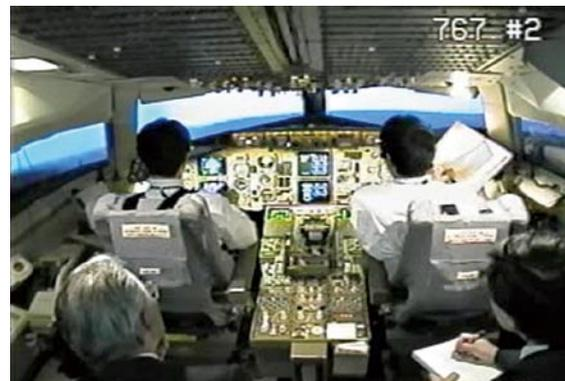
Fig. 3 Simulated line-oriented flight training
