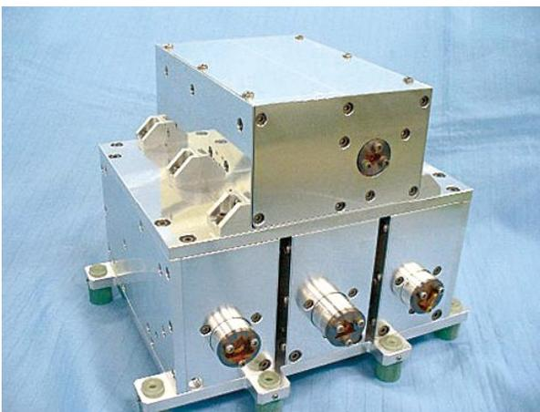
Fig.3 Photograph of JASON-2 LPT sensors
