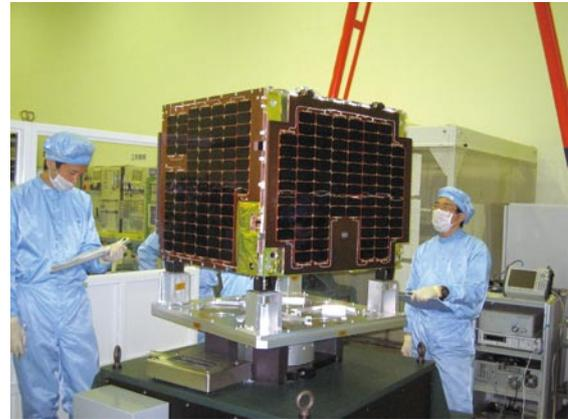
Fig.4 Mass balance test of SDS-1 flight model
