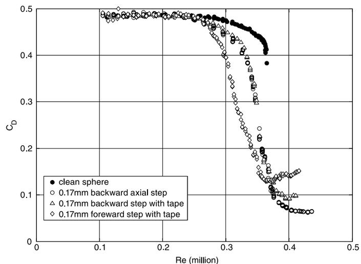
Fig.1(b) The Reynolds number effect on spheres with varying roughness.
