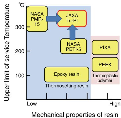
Fig.3 Newly developed polyimide resin has an 80K higher temperature capability and superior mechanical properties, with triple the strength and 10 times the tensile failure strain compared to existing heat resistant materials
