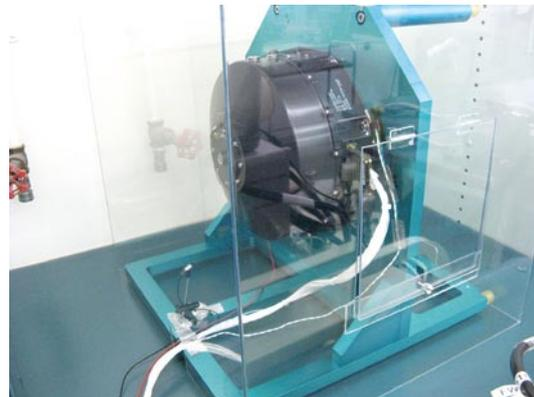
Fig. 2 High-performance reaction wheel long-term operation test
