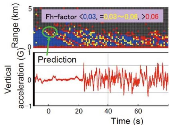
Fig.7 Intensity prediction for possible severe turbulence
