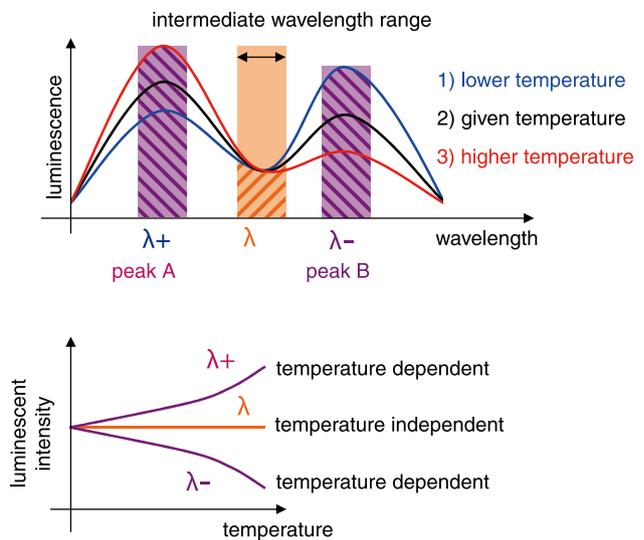
Fig.2(a) Temperature-cancellation method using two luminescent peaks.
