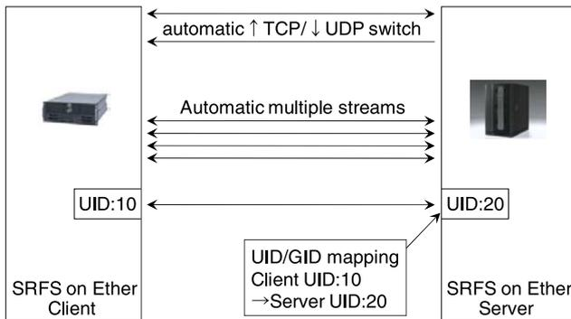
Fig.5 "SRFS on Ether" features
