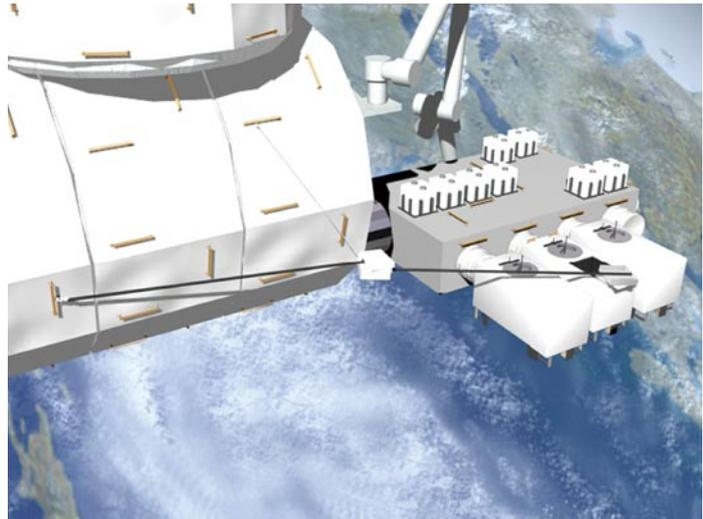
Fig.5 An artist's image of the robot system in REX-J moving along the surface of KIBO using tethers
