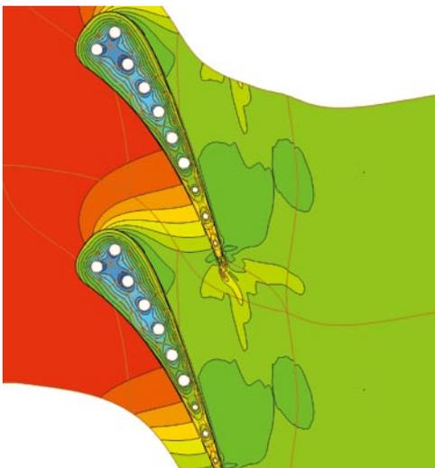
Fig.9 Conjugate flow and heat transfer simulation of turbine cross section
