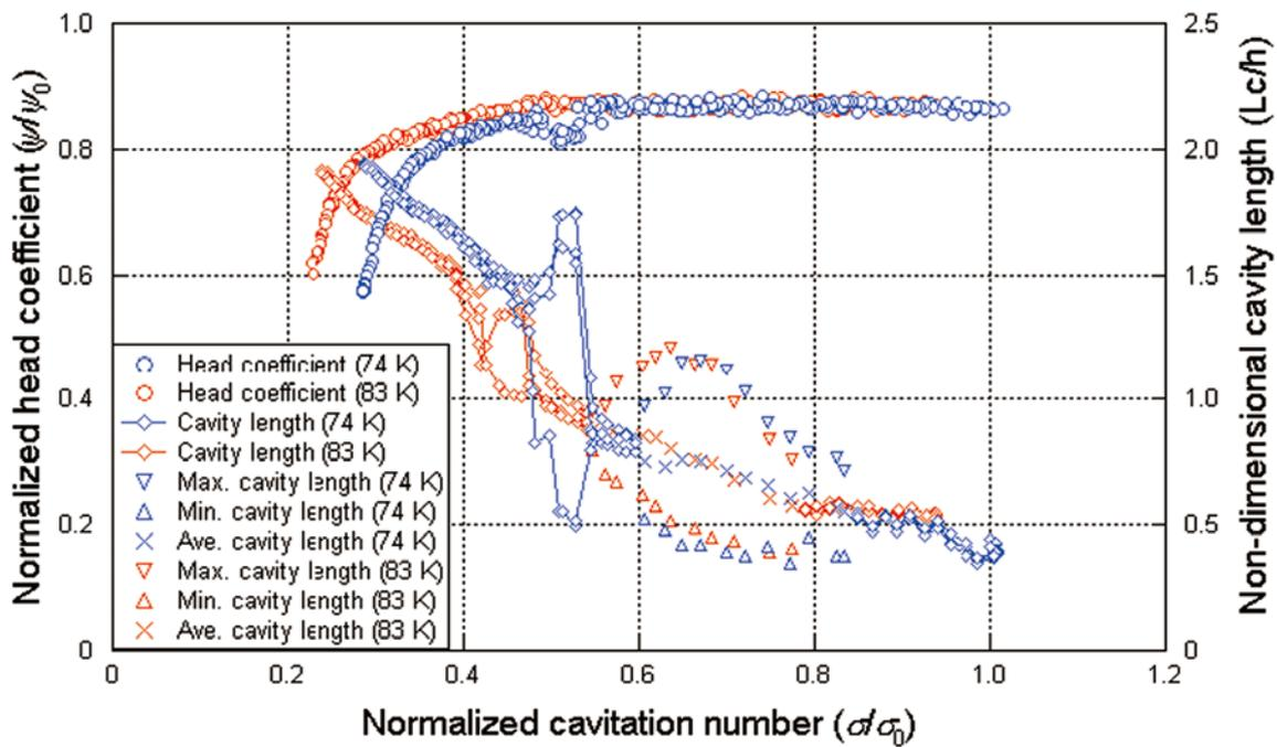
Fig.3 Cavitation performance and cavity length at 74 K and 83 K
