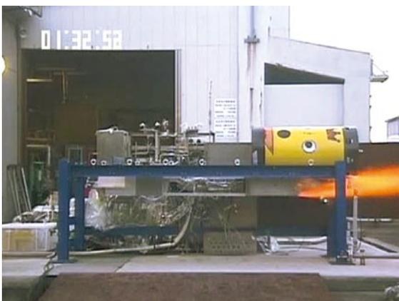
Firing Test at Sea Level Condition
