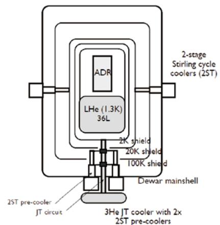
Fig.3 Cooling system design for ASTRO-H/SXS
