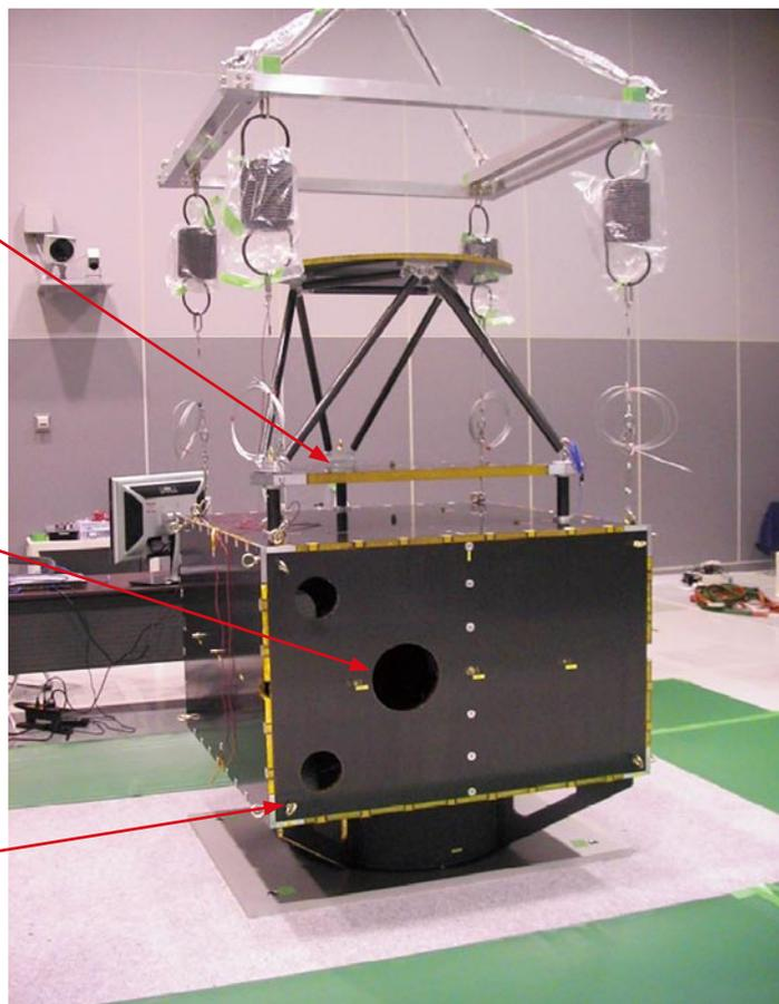
Fig.2 Satellite Structure Model Suspended in Midair by Springs for Microvibration Transmission Measurement
