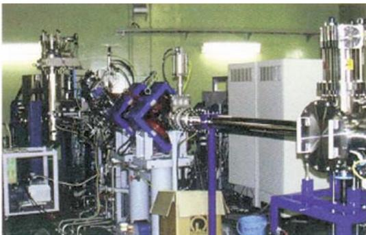
Fig.2 Irradiation equipment for single-event evaluation(At the Takasaki Research Institute of the Japan Atomic Energy Agency)
