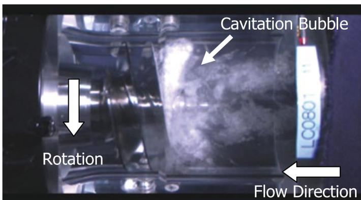
Fig.5 Turbopump inducer cavitation test
