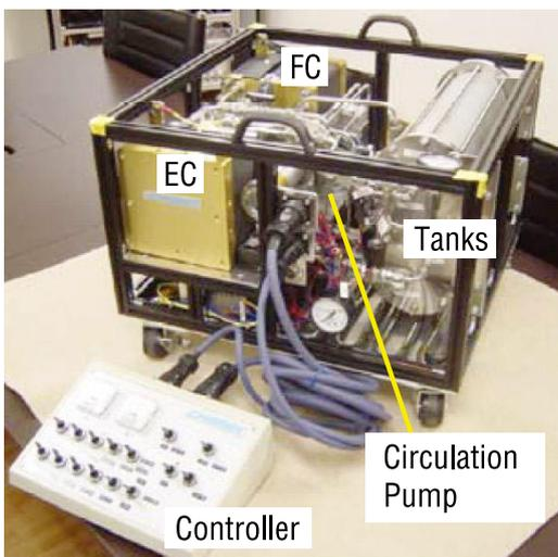
Fig.8 Breadboard model (BBM) of regenerative fuel cell system
