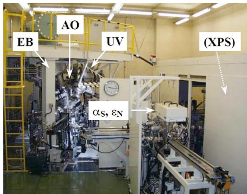
Fig.5 Combined space environment test machine
