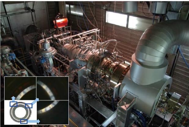
Fig.6 Test section of annular combustor test facility (Flame in combustor at the lower left)
