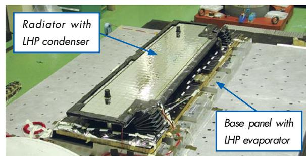
(b) Deployable Radiator (DPR) with LHP onboard ETS-VIII
