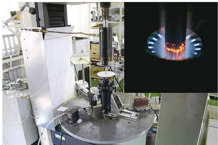
Fig.10 Burner test rig for superalloy evaluation
