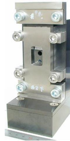
Fig.2 Proposed test fixture for the open hole compression (OHC) test - This test fixture allows the use of a much smaller test specimen than the conventional test configuration.
