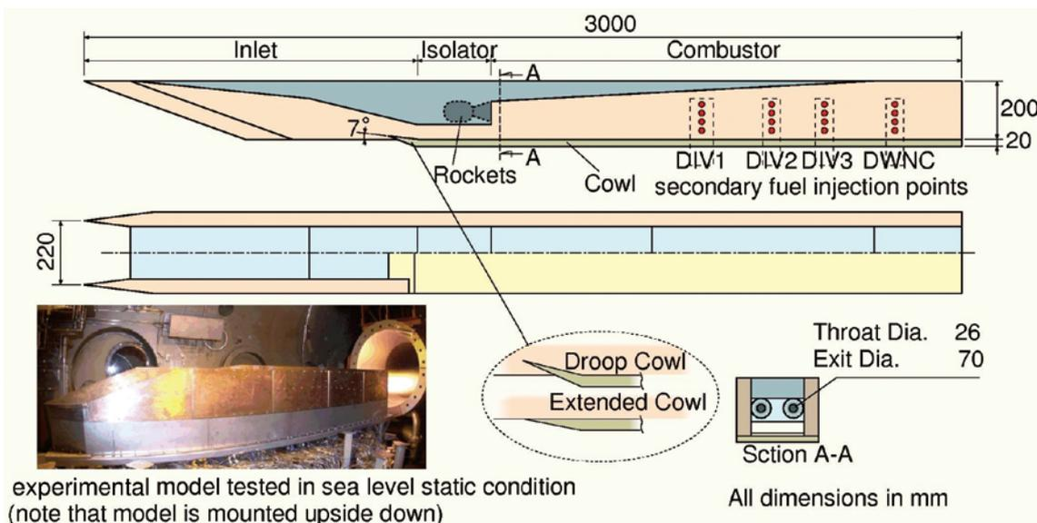
Fig.2 Schematic view of the combined cycle engine experimental model
