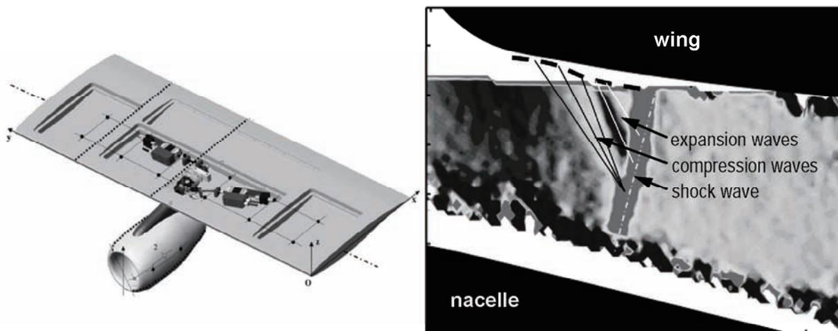
**Figure 4** Research project WIONA: sketch of the model with excitation system (left) and PIV-evaluated, streamwise development of mechanical energy for the maximum downstream shock location
