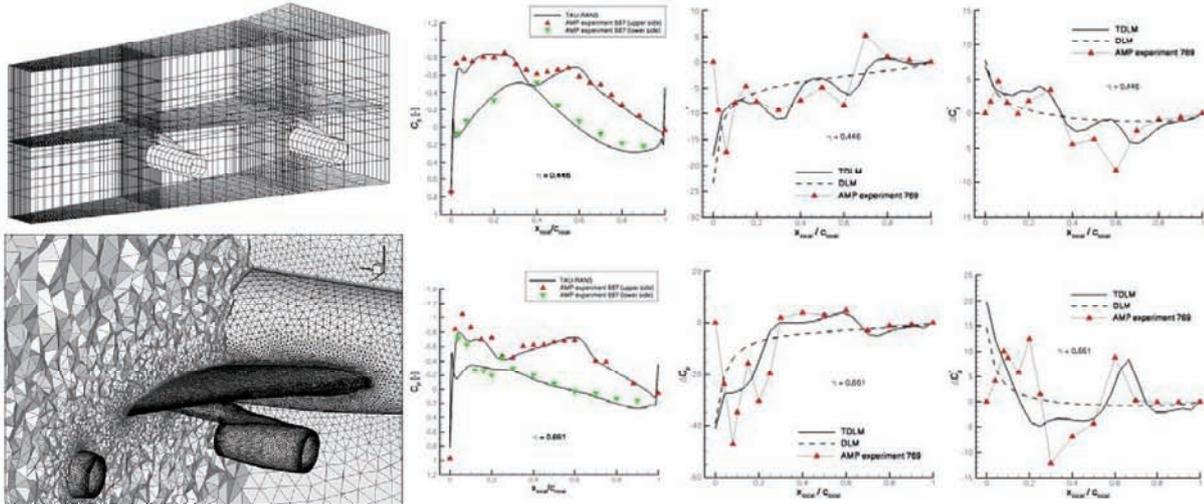
**Figure 5** Unsteady  $C_p$  distribution (real and imaginary components) for AMP WBPN model comparing TDLM and steady RANS results with experimental data (pure pitching motion,  $\omega^*=0.369$ ,  $Ma=0.820$ ,  $\alpha=1.80^\circ$ ,  $Re=3.57 \cdot 10^6$ )
