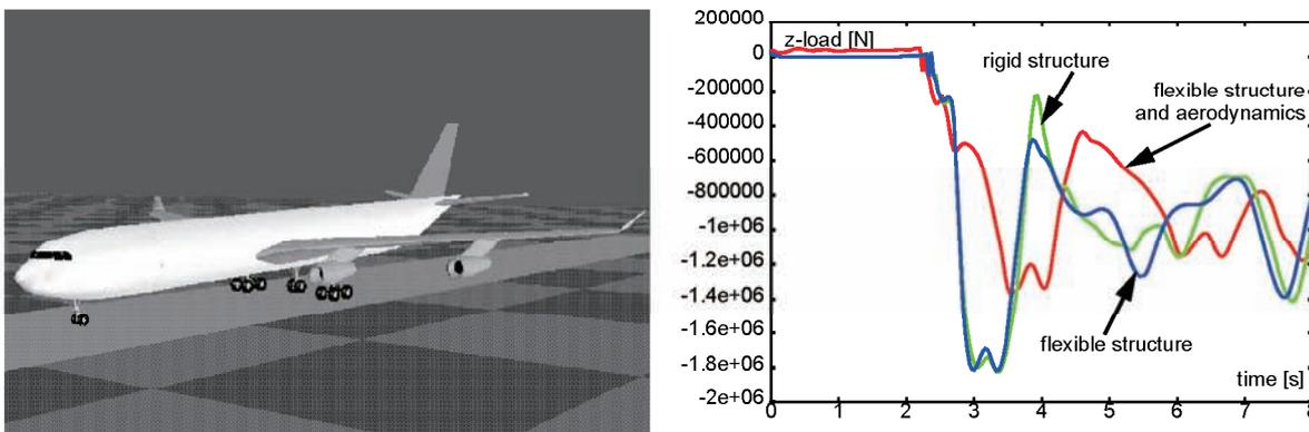
**Figure 6** *Multibody simulation of the touch-down of a large transport aircraft (left), vertical load on the main landing gear leg attachment (right) comparing: certification requirement (rigid airframe), industry standard (flexible airframe) and including aerodynamic effects of airframe deformation (flexible and aerodynamics)*
