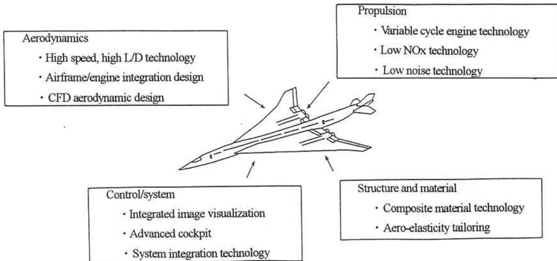
Fig. 6 Key technologies for R & D of SST
