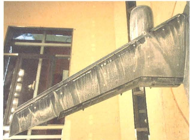
(a) Oil-flow visualization (60m/s, \text{AoA}=15^\circ )
