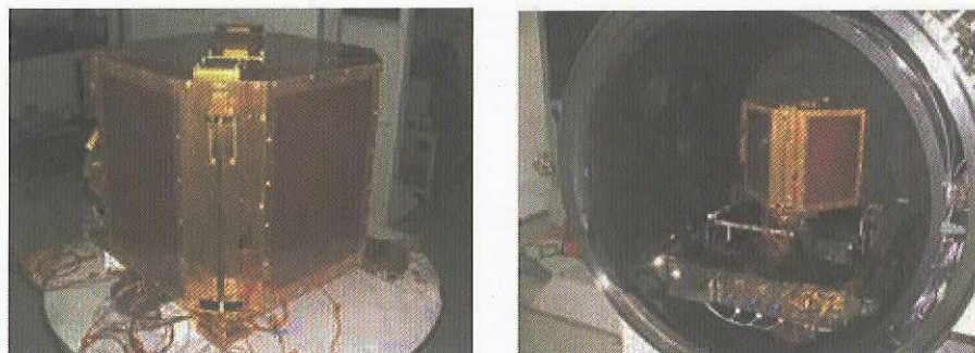
Fig.4 STM of SOHLA-1 for Thermal Balance Test
