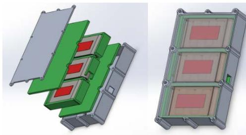
**Figure 4 CAD design of battery box**
