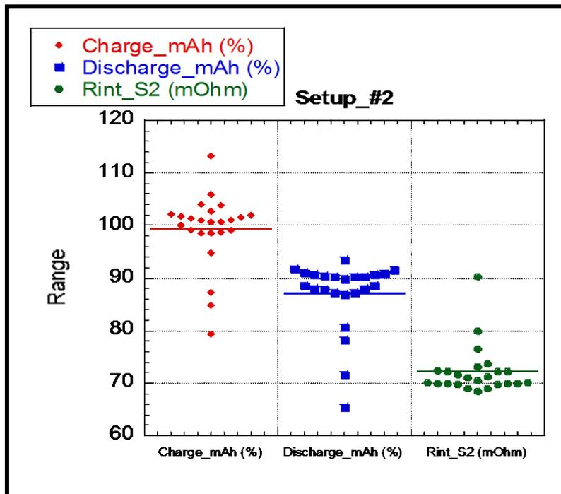
Figure 12 Range of variation of the Charged /discharged capacity and internal impedance of the cells screened by setup2
