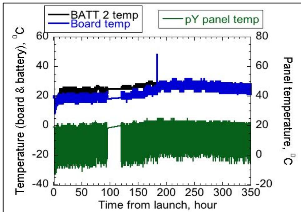
Figure 18 Battery temperatures on orbit, °C
