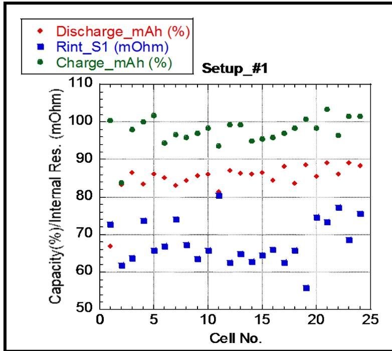
Figure 11 Charged /discharged capacity and internal impedance versus cell numbers screened by setup1
