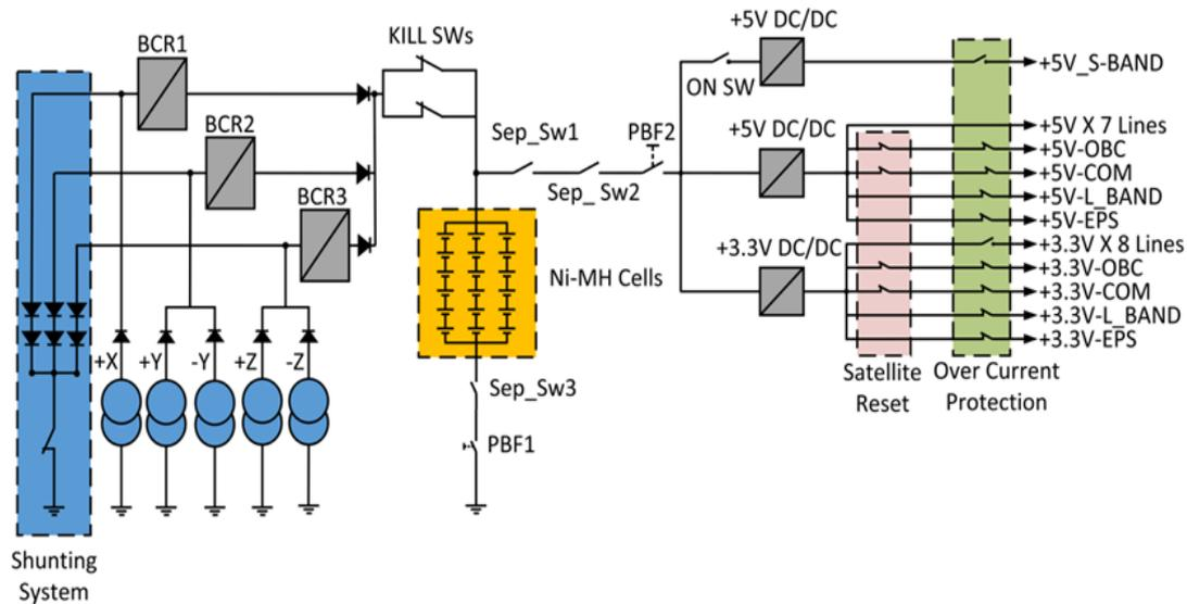
Figure 1 HORYU-IV Electrical Power Subsystem Block diagram [1]
