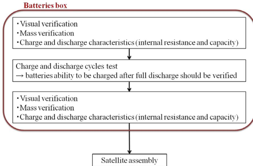
**Figure 3 Battery Box assembly requirements**
