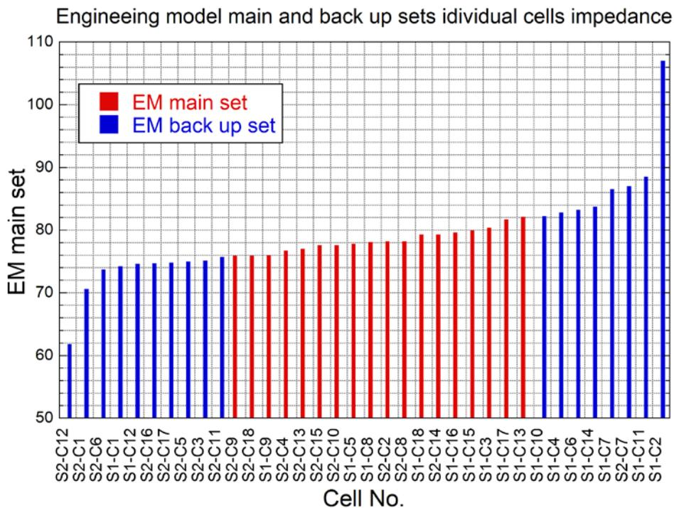
**Figure 9 Engineering model main and back-up sets individual cells impedance**
