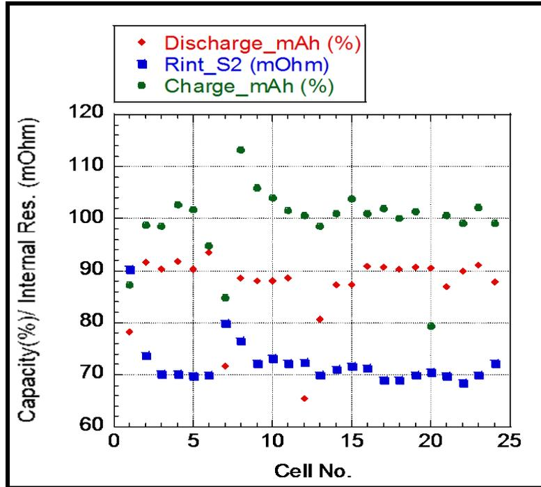
Figure 13 Charged /discharged capacity and internal impedance versus cell numbers screened by setup2
