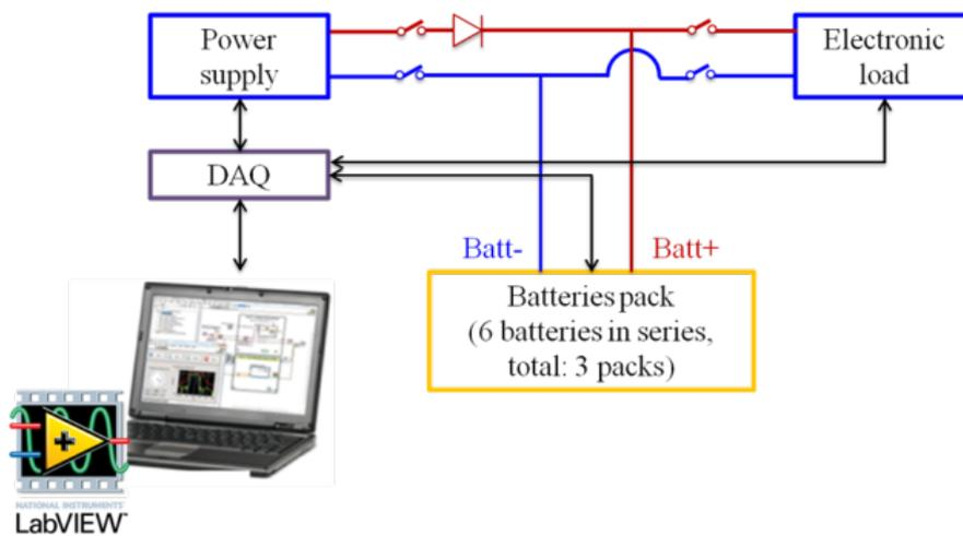
Figure 6 Block diagram of measurement setup (setup1 and setup2)
