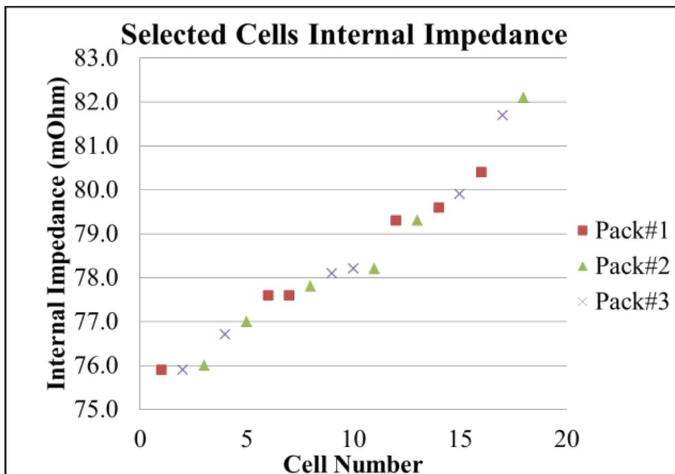
Figure 14 Selection cells internal impedance for corresponding packs
