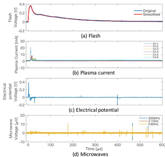
Fig 5. Comparison of each electrical phenomenon.
