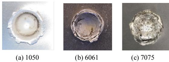
Fig. 3. Craters of the impacted targets.
