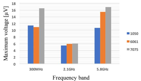
Fig. 7. Comparison of maximum amplitude of microwaves depending on target materials.
