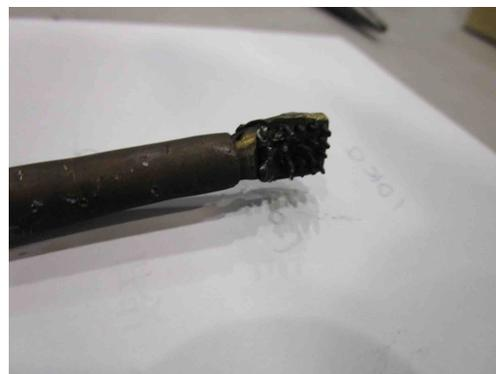
Fig. 3. A photograph of the 16-ch Langmuir probe array, which is set in the pressurized chamber.
