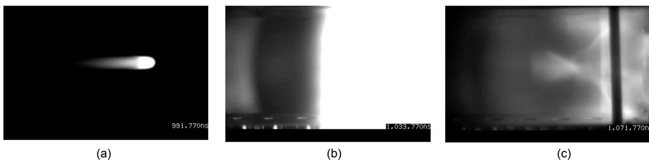
Fig. 4. Profile images in front of the entrance orifice. The right end is the entrance surface. (a) The projectile is coming at speed of 7 km/s. (b) Strong emission from the gas plume. (c) The cloud of carbon particles coming out with speed of about 1 km/s.
