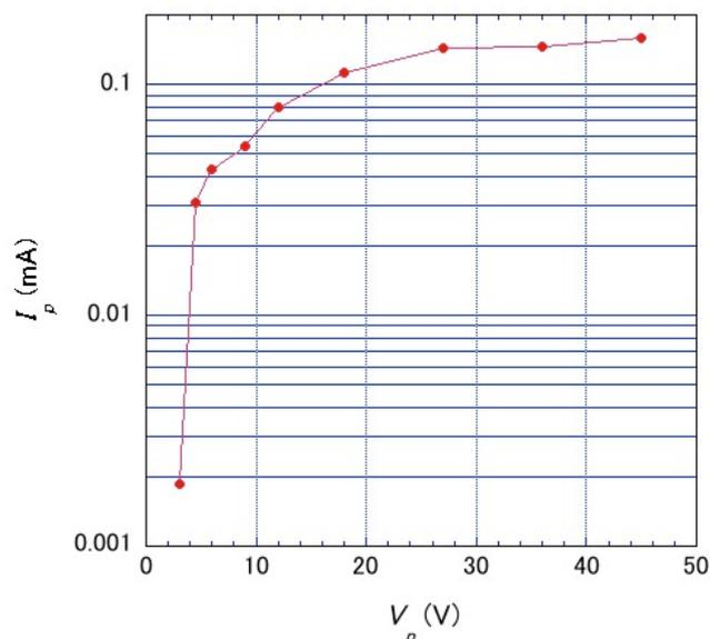
Fig. 5. A typical I-V characteristic of the probe measurement when the gas plume flows over the probe.
