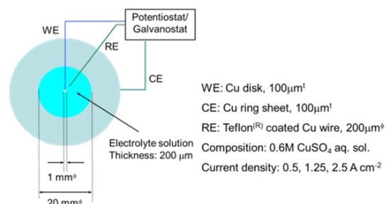
Fig.1 Schematic illustration of quasi-two dimensional electrolytic cell.
