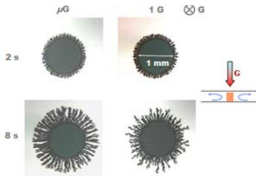
Fig.3 Morphological variations of electrodeposited copper;  $i=2.5 \text{ A cm}^{-2}$
