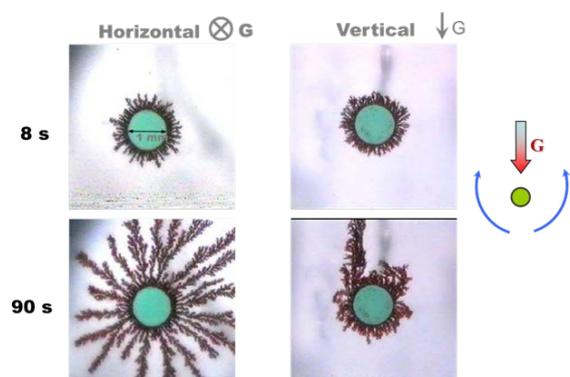
Fig.2 Morphological variations of electrodeposited copper;  $G=1 \text{ G}$ ;  $i=2.5 \text{ A cm}^{-2}$
