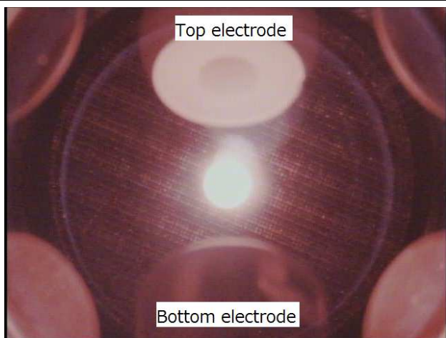
Fig.4 A molten alumina sample levitated in the ISS-ELF
